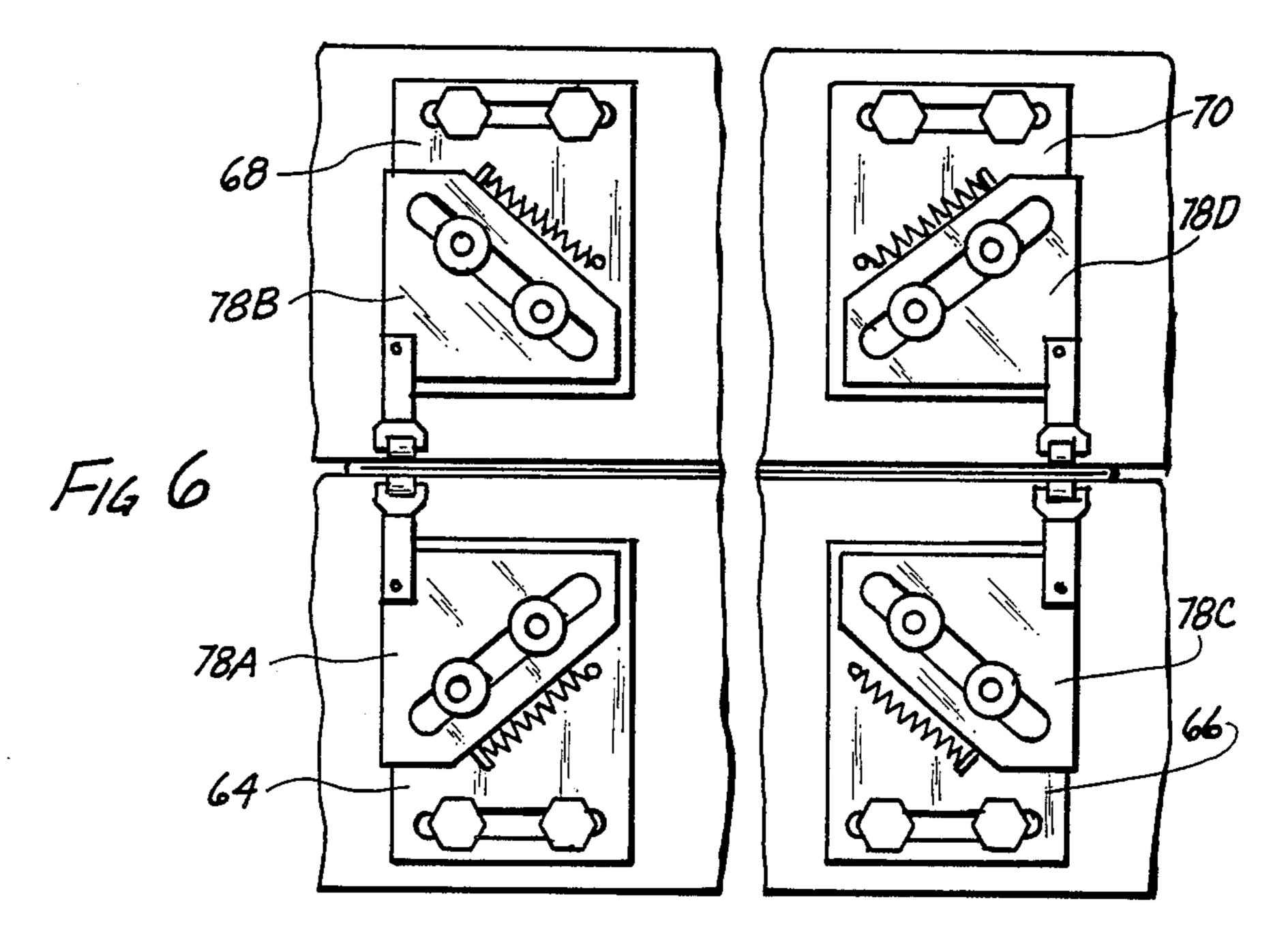
BAG GRIPPER AND SPREADER FOR FORM, FILL AND SEAL BAGGING MACHINE
