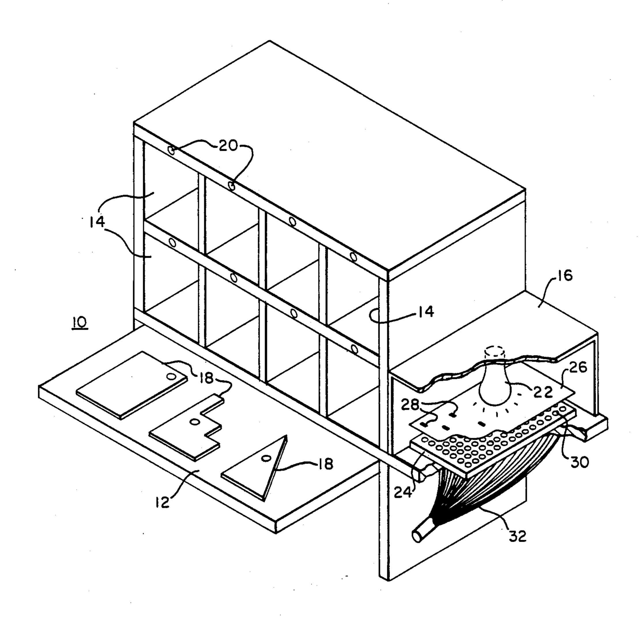
to indicate to an assembly operator which parts to select for assembly of a particular workpiece.
