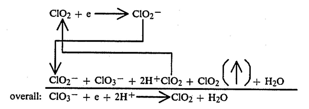
From these equations, it will be seen that the process can be considered autocatalytic, in that generated chlorine dioxide is used to produce the active species for reduction of chlorate ions. A residual concentration of chlorine dioxide must be maintained in the aqueous acid solution to sustain the autocatalytic cycle.
