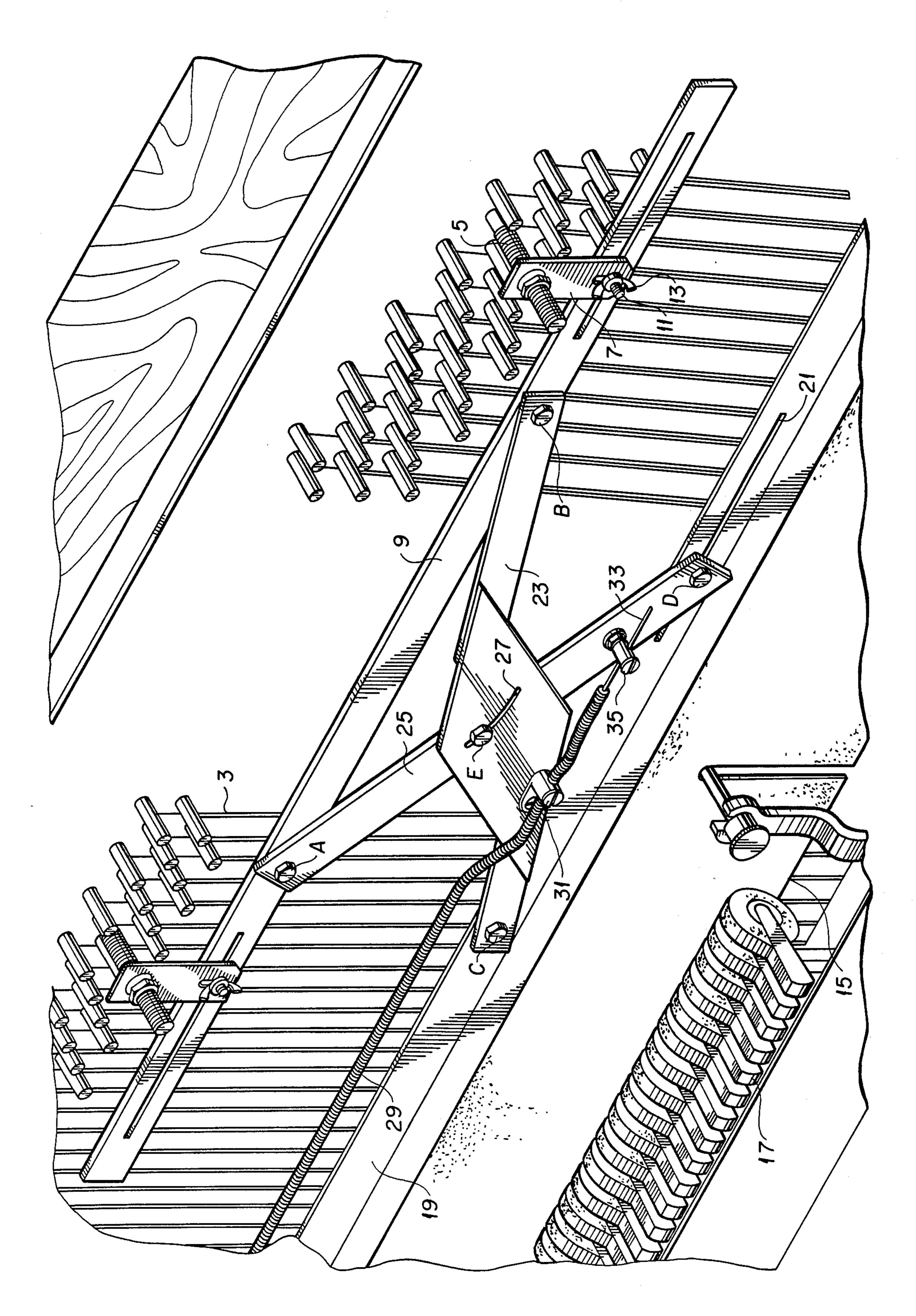
(9) by way of a bolt (11) capable of sliding along the associated grooves and able to be easily tightened by way of a winged nut (13).
