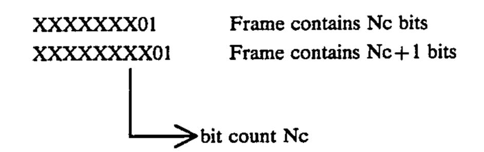
Consequently, when Nc bits have been counted from the beginning of the preceding flag, the two next bits including the first bit of the flag and the additional bit of the frame, if any, cannot simulate the 01 delimiting pattern whatever the value of this additional frame bit can be. When Nc bits have been counted, the detection of the 01 pattern indicates that the frame contains Nc bits.
