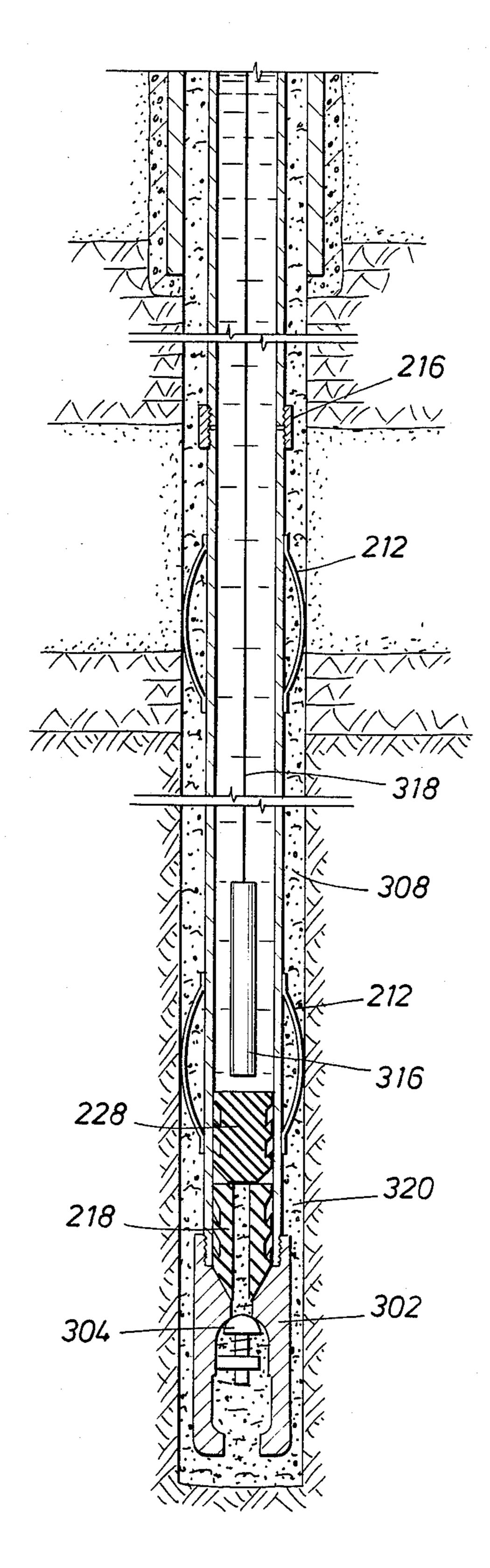
METHOD FOR PRIMARY CEMENTING A WELL WITH A DRILLING MUD WHICH MAY BE CONVERTED TO CEMENT USING CHEMICAL INITIATORS WITH OR WITHOUT ADDITIONAL IRRADIATION
