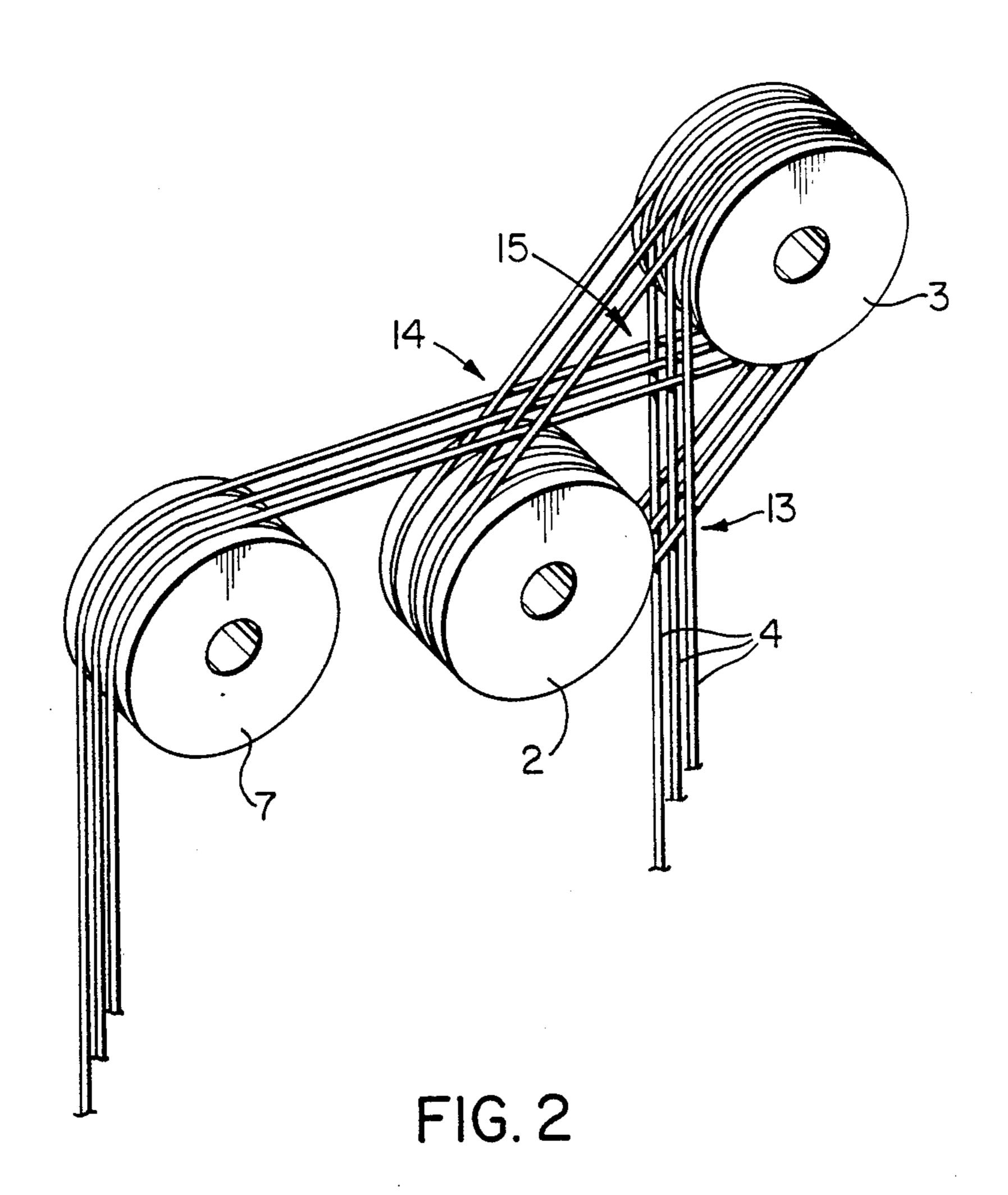
ELEVATOR WITH TRACTION SHEAVE
