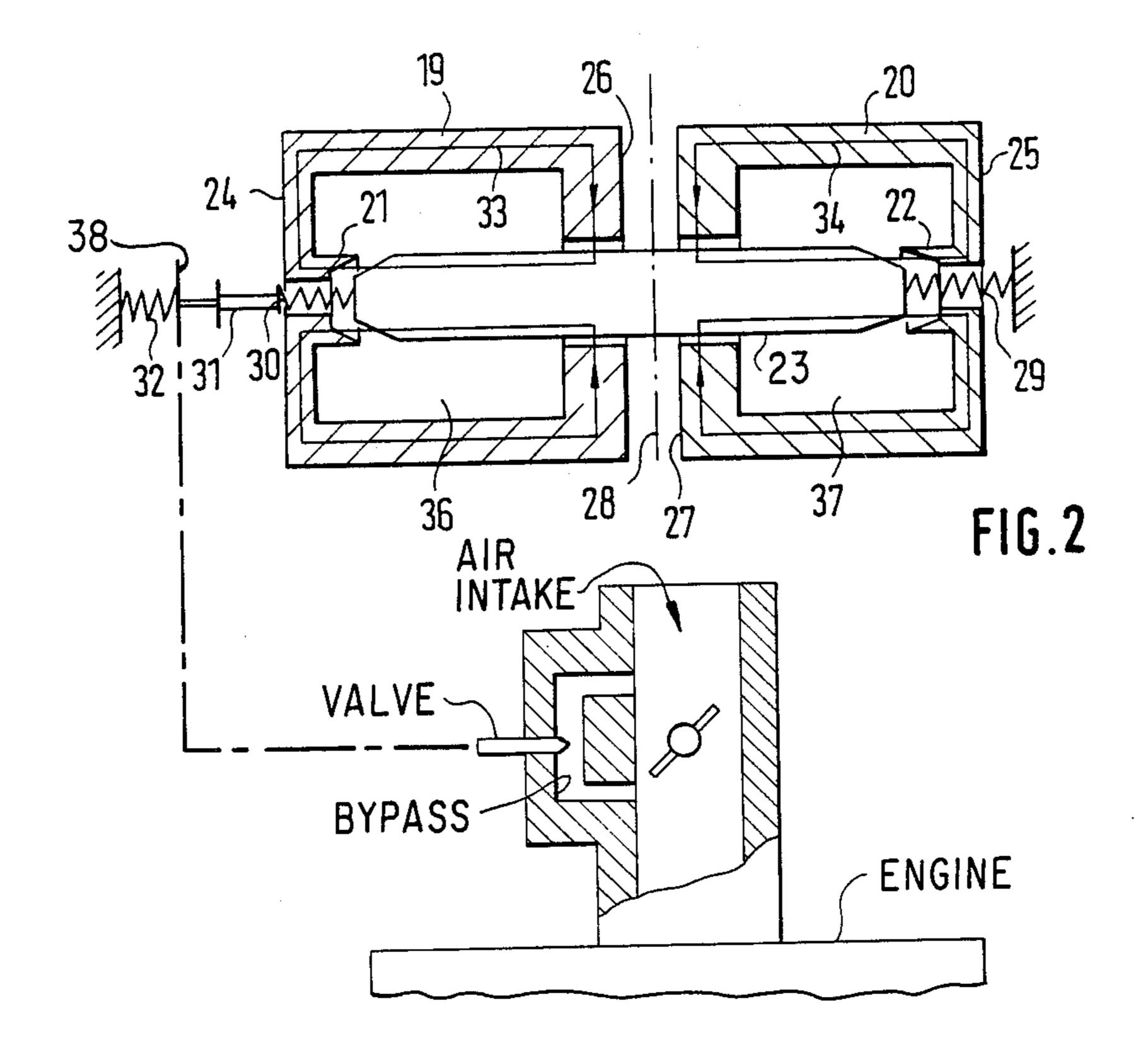
DEVICE FOR REGULATING THE IDLING SPEED OF AN INTERNAL COMBUSTION ENGINE
