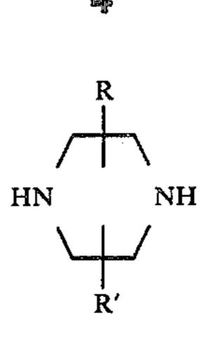
wherein R and R' represent each a hydrogen atom or a hydrocarbon residue of 1-4 carbon atoms, in an amount of 0.15 equivalent or more as stoichiometrically calculated based on the epoxy equivalent of the emulsion or suspension of the epoxy compound.
