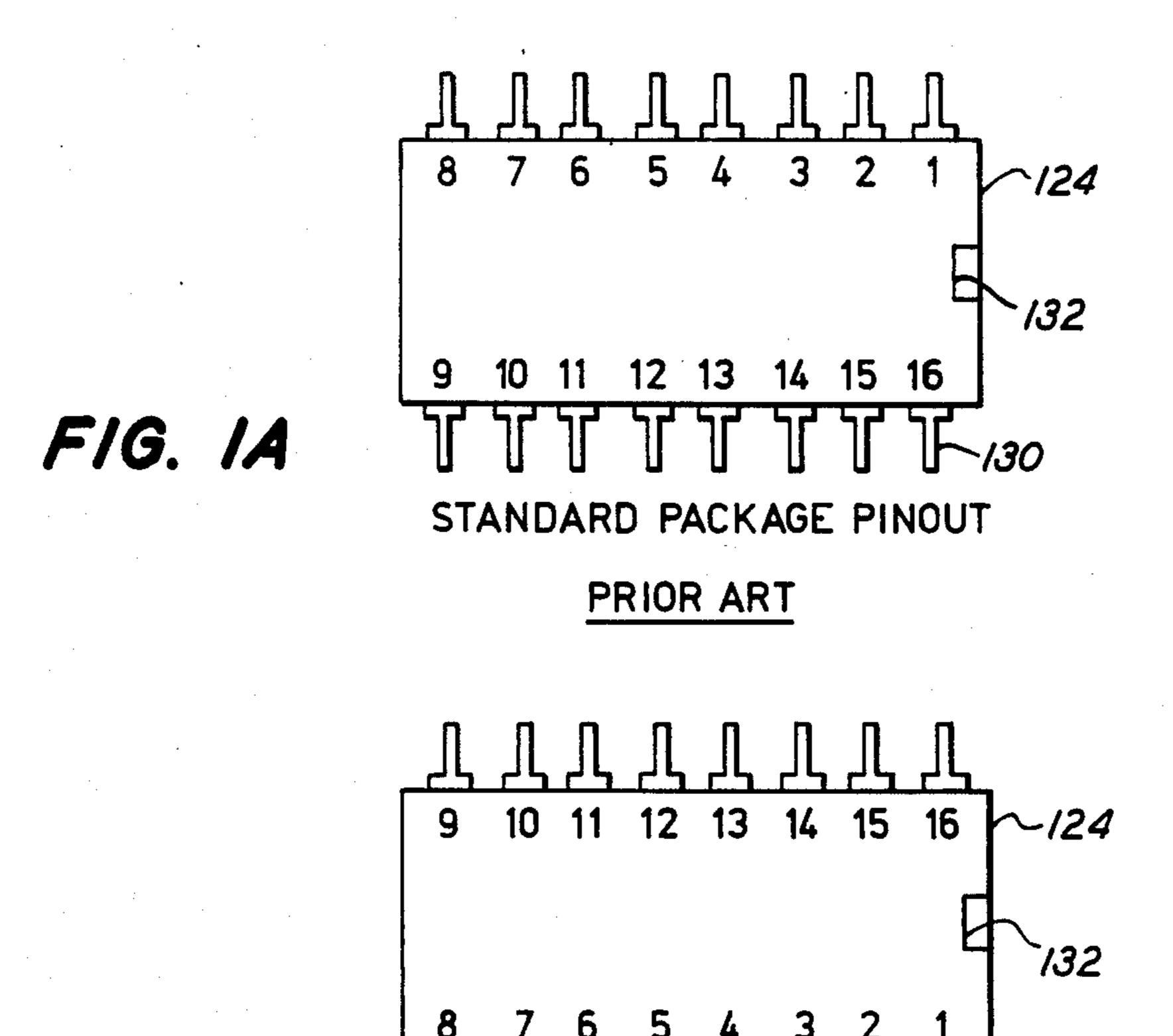
INVERTED PACKAGE PINOUT
