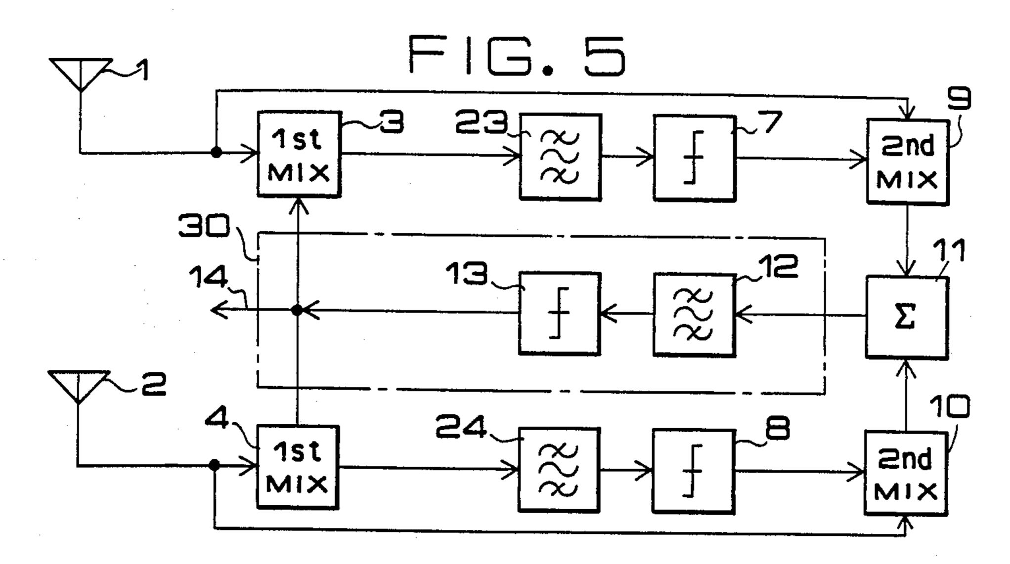
1,2: RECEIVING ANTENNA 30: FEEDBACK CIRCUIT
