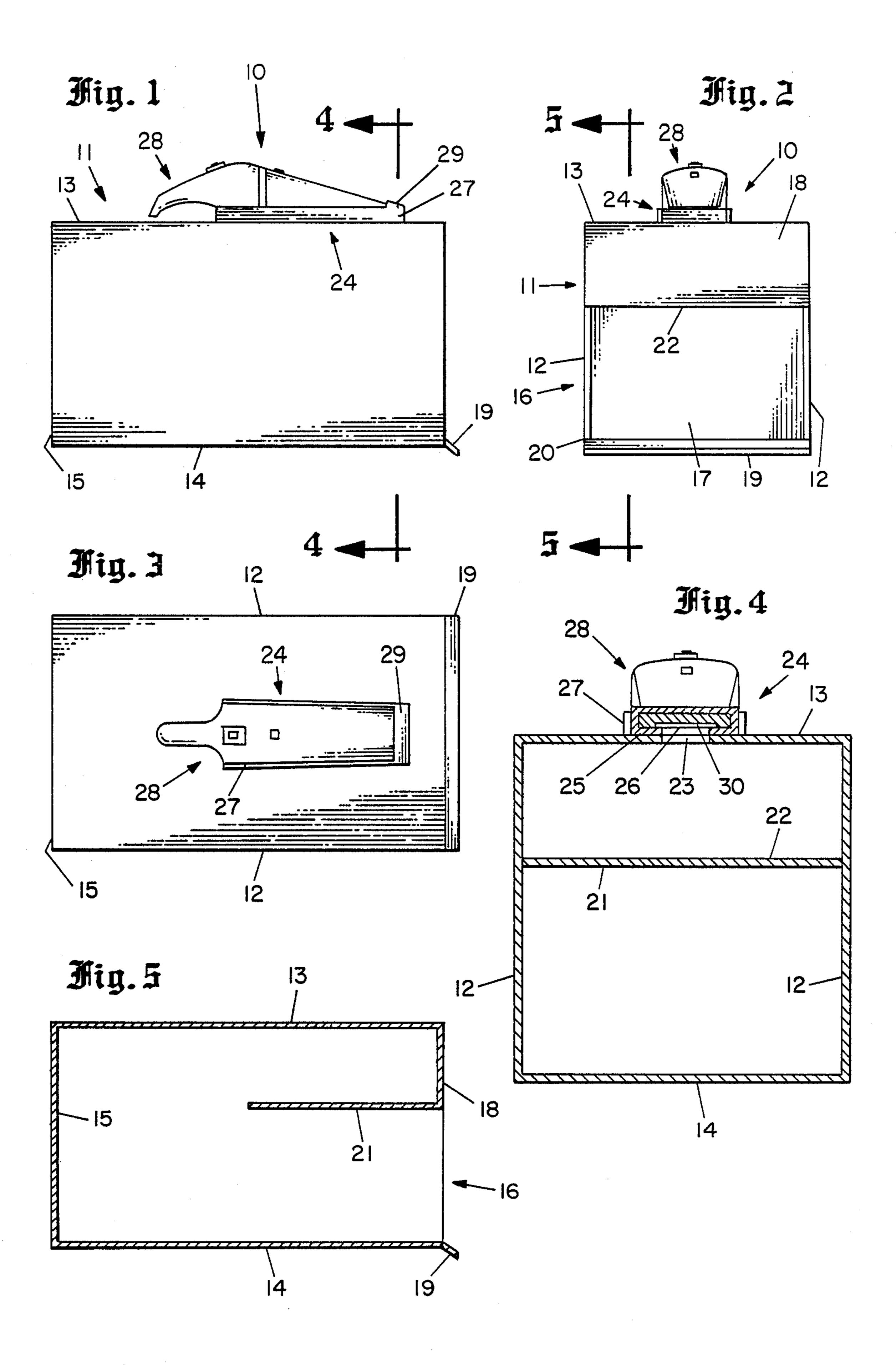
FIG. 4, is an enlarged interior view of FIG. 1, taken along line 4—4, and
