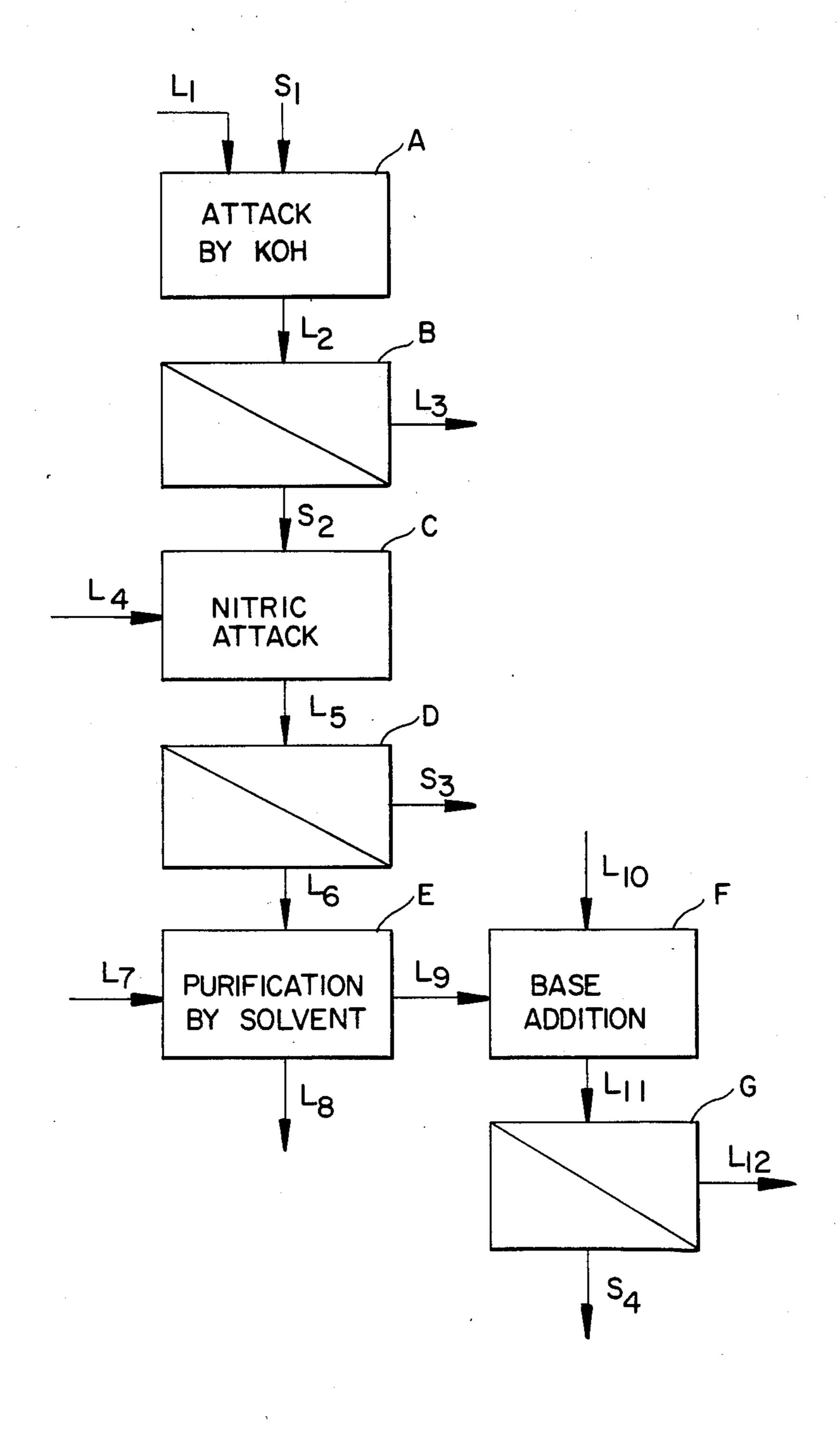
PROCESS FOR THE SEPARATION OF RARE EARTHS AND URANIUM OF A UF<sub>4</sub> CONCENTRATE AND FOR PUTTING THEM INTO USEFUL FORM
