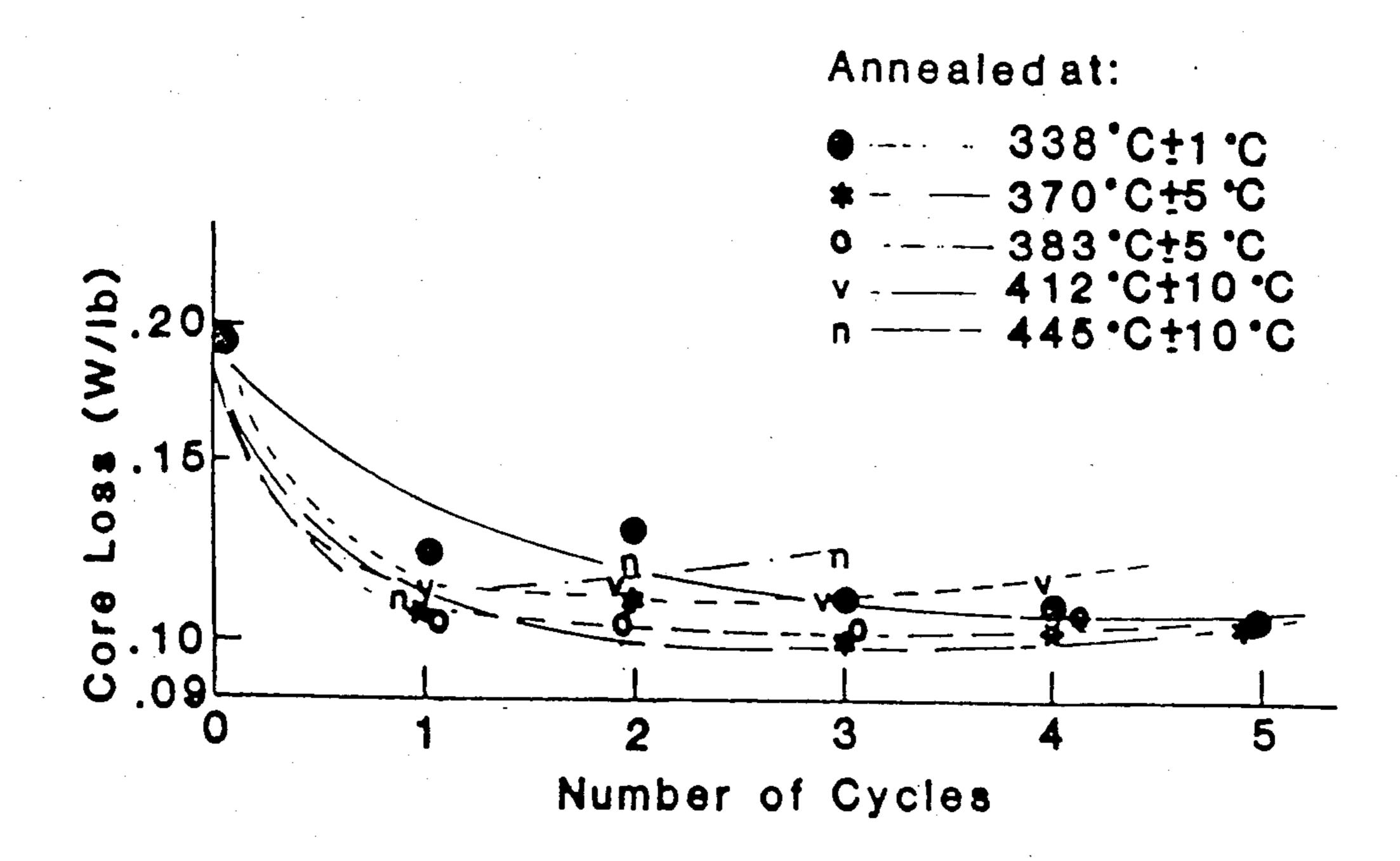
Figure 2. Core Loss at 14 kG Versus Number of Heating Cycles for Amorphous Metal Strips Annealed in a Conveyor Furnace.
