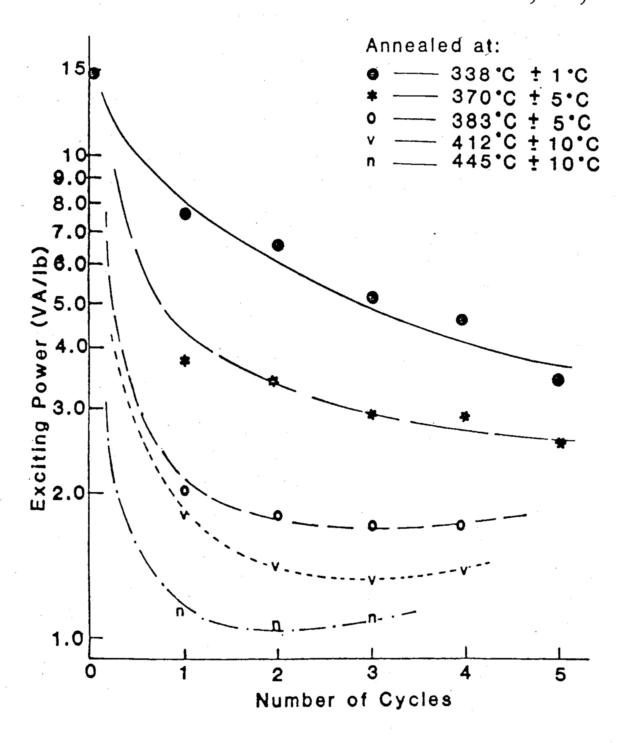
Figure 3. Exciting Power at 14 kG Versus Number of Heating Cycles for Amorphous Metal Strips Annealed in a Conveyor Furnace.
