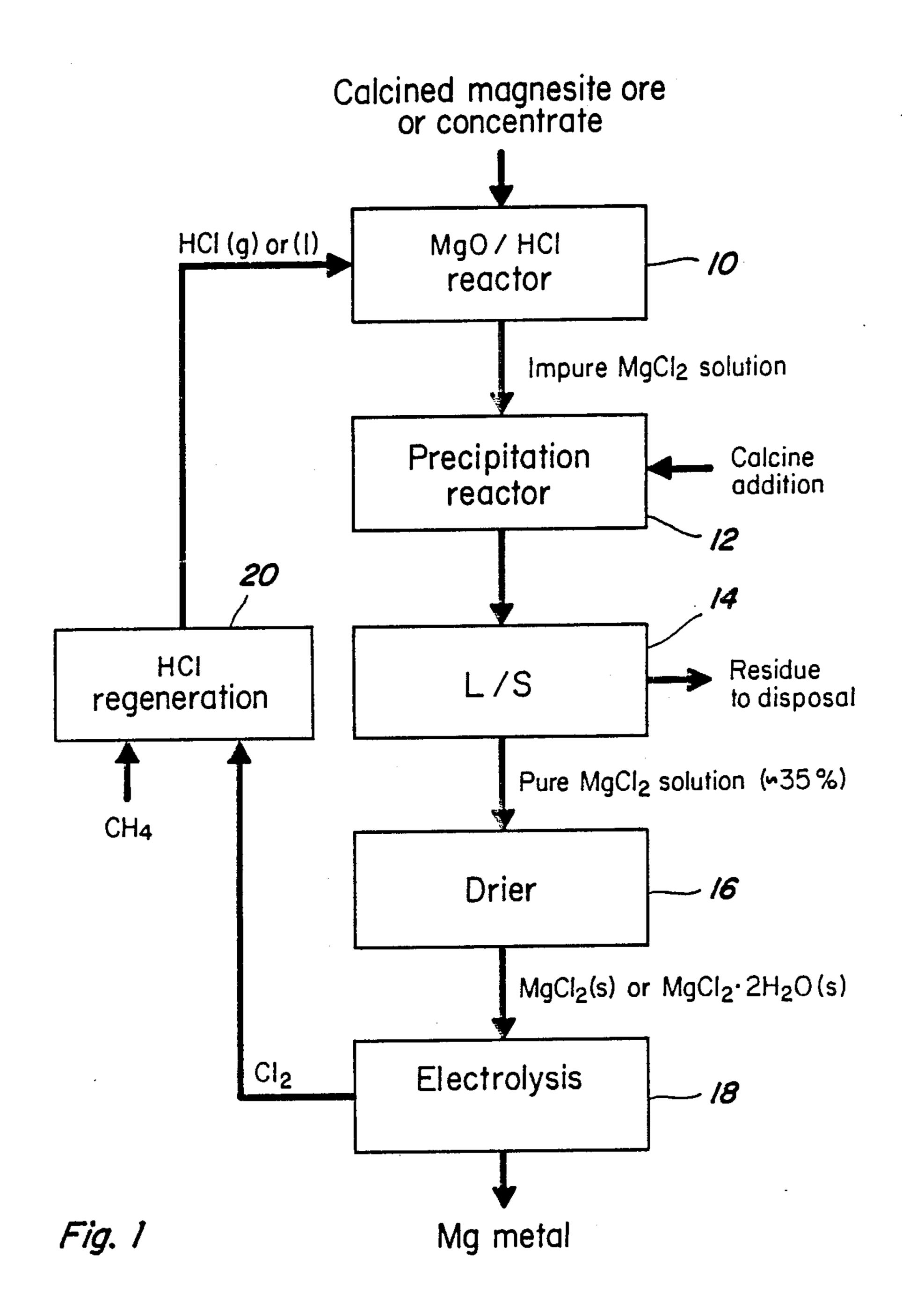
PRODUCTION OF PURE MGCL<sub>2</sub> SOLUTION SUITABLE FOR THE PRODUCTION OF MAGNESIUM METAL FROM AN IMPURE MAGNESITE ORE OR CONCENTRATE
