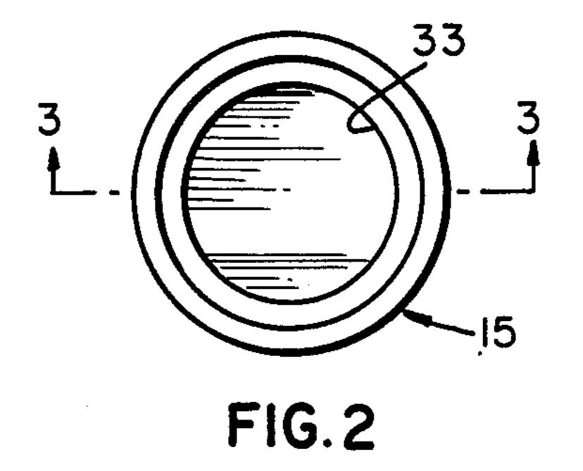
end and a cap 15 is positioned at the rearward end for retaining the bit 11 in the bore 17 of the bit holder 13.
