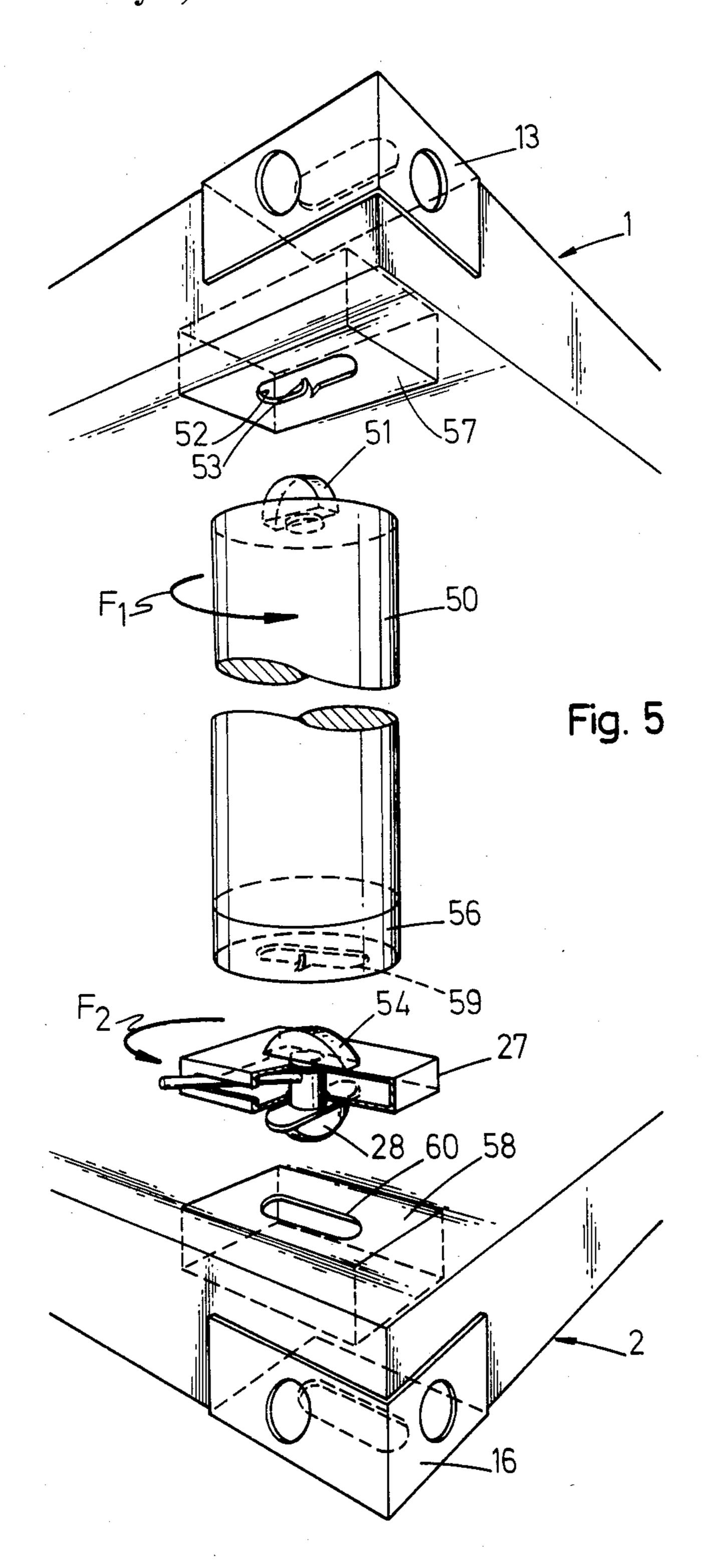
CONTAINER SHAPED STRUCTURAL ELEMENT AND STRUCTURE OBTAINED FROM A PLURALITY OF COMPONENTS FROM SUCH CONTAINERS
