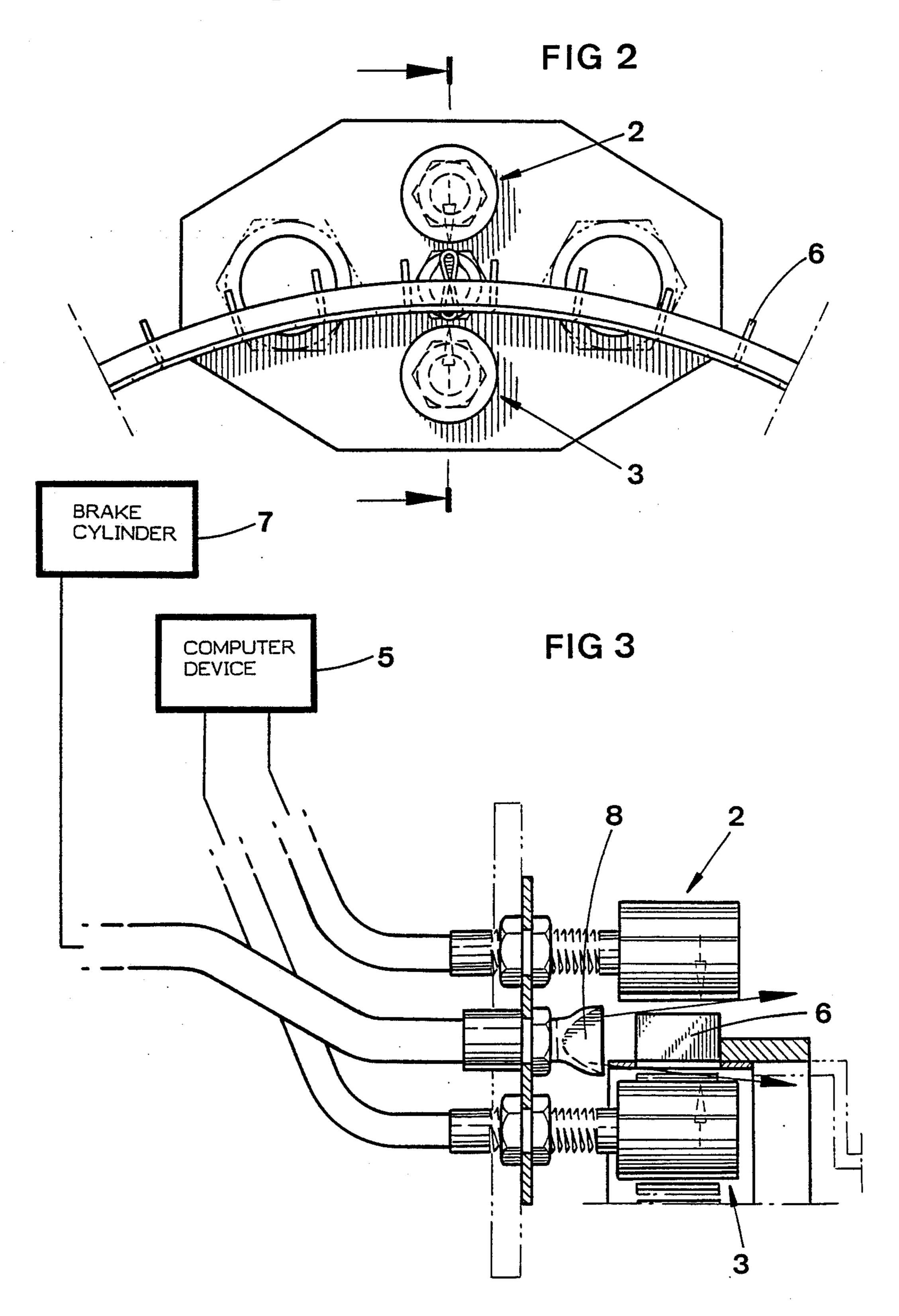
ARRANGEMENT FOR AN OPTICAL SPEED INDICATOR
