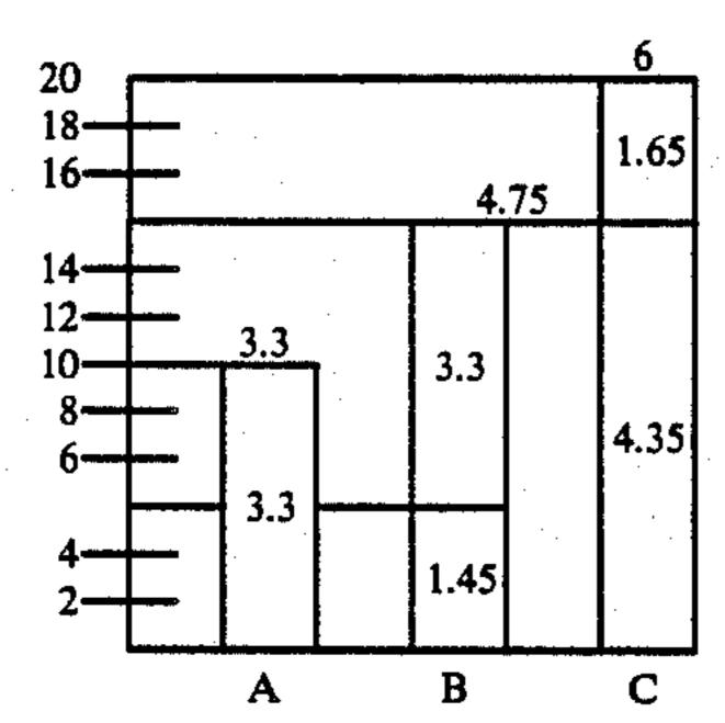
Composition A refers to the case where to the front face is bonded a metal sheet whose thickness is between 1 and 1.2 mm and composition B relates to the case where there is bonded to the front face a metal sheet whose thickness is between 0.5 and 0.7 mm, whereas composition C is relative to the absence of a metal sheet on the front face.
