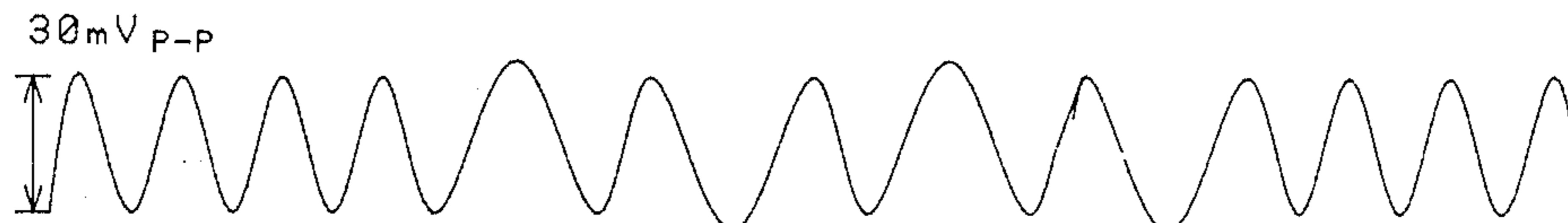
RECEIVED SIGNAL, 6000' ALONG THE CABLE, DIFFERENTIATED.
