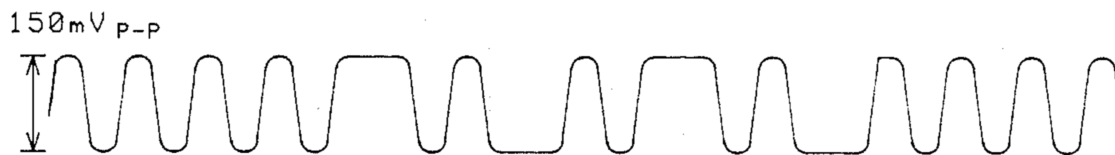
RECEIVED SIGNAL, 4000' ALONG THE CABLE, DIFFERENTIATED.
