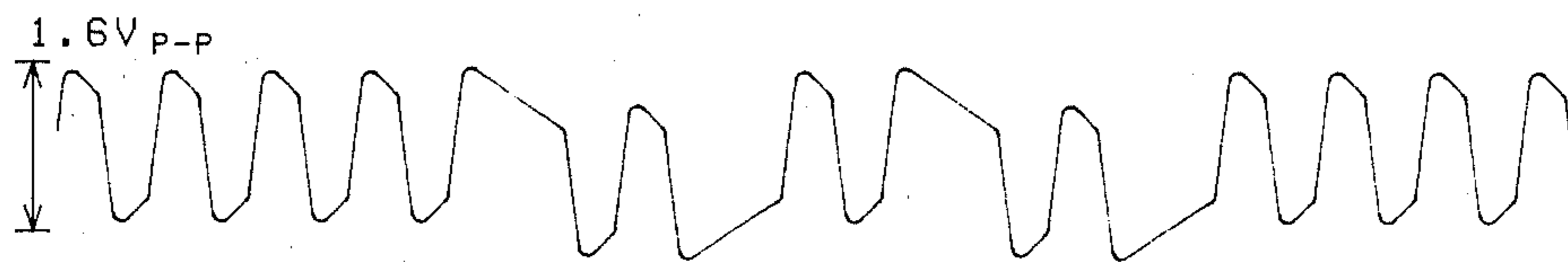
RECEIVED SIGNAL, 1000' ALONG THE CABLE, DIFFERENTIATED.
