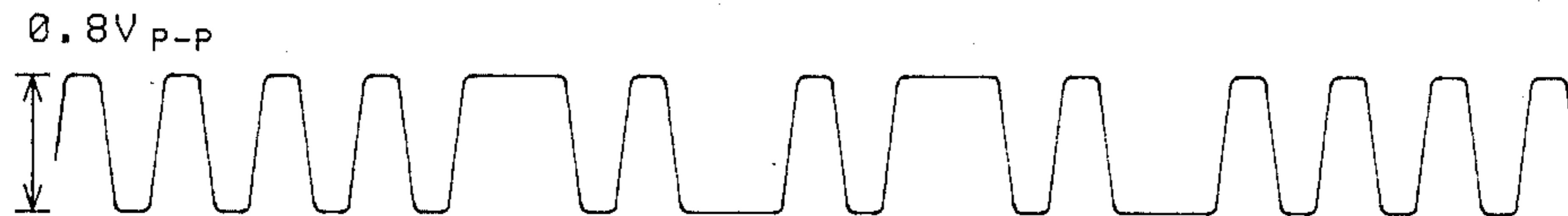
RECEIVED SIGNAL, 2000' ALONG THE CABLE, DIFFERENTIATED.
