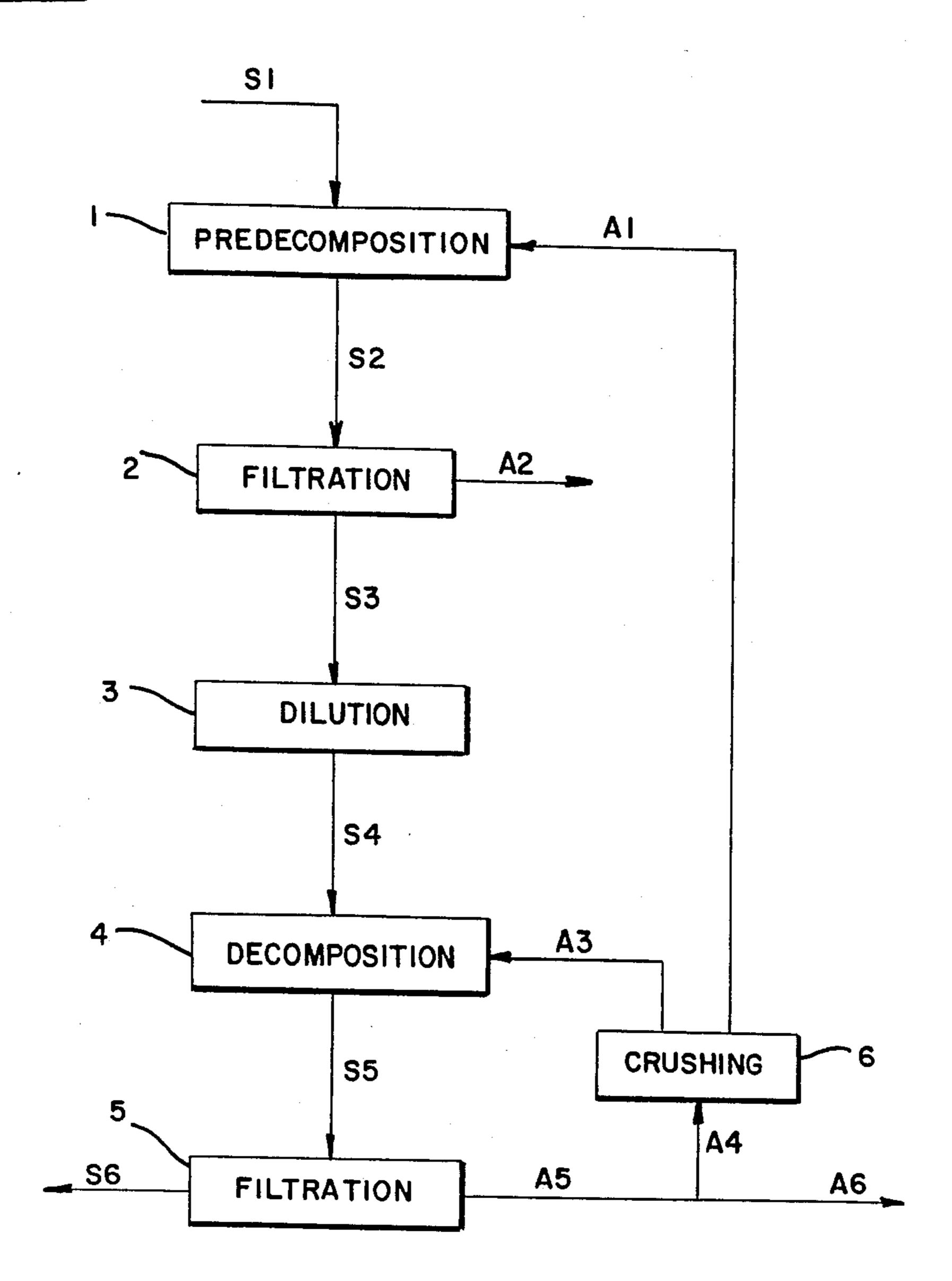
PROCESS FOR THE PRODUCTION AT A HIGH LEVEL OF PRODUCTIVITY OF ALUMINUM TRIHYDROXIDE IN A HIGH STATE OF PURITY AND WITH A MEDIAN DIAMETER OF LESS THAN 4 MICROMETERS, WHICH IS REGULATED AS REQUIRED
