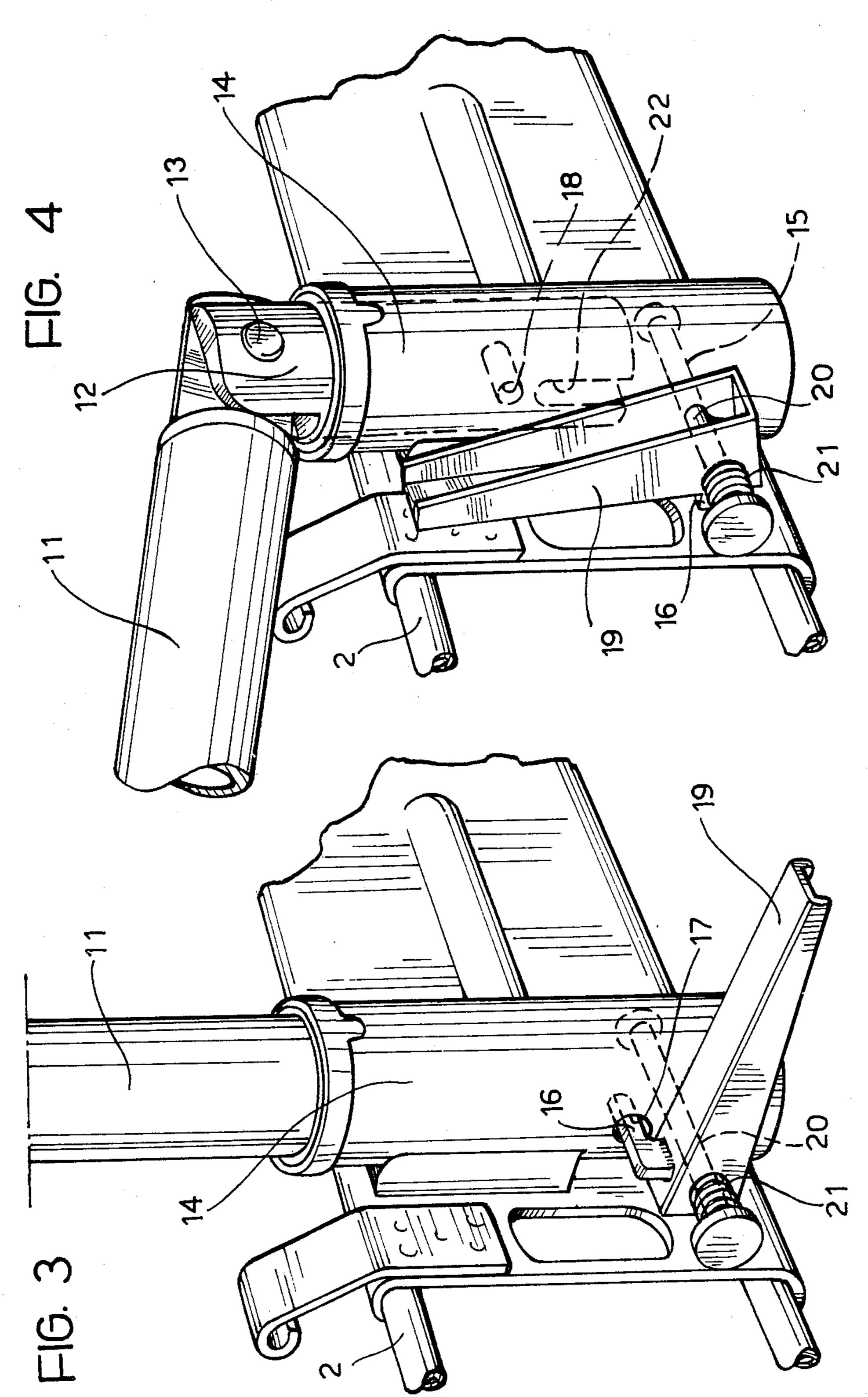
The support 9 is constituted by two spaced-apart pillars 11 each of which has a lower end portion 12 (FIGS. 2 and 4) jointed about a transverse articulated pin 13.
