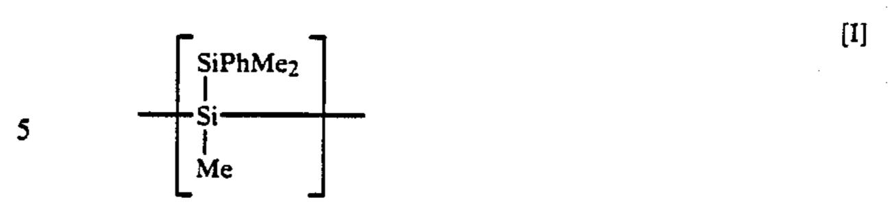
wherein, Ph is phenyl, and Me is methyl, and has a weight average molecular weight in the range of from 5,000 to 500,000.
