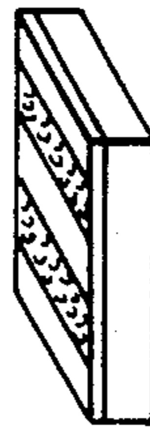
FIG. 3f RESIST STRIPPED
