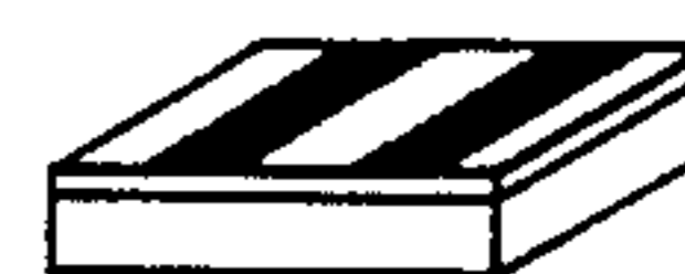
CONDUCTIVE COPPER TRACKS DYED BLACK AND PROVIDED WITH A PROTECTIVE COATING
