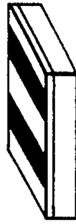
FIG. 3g CONDUCTIVE COPPER TRACKS DYED BLACK AND PROVIDED WITH A PROTECTIVE COATING
