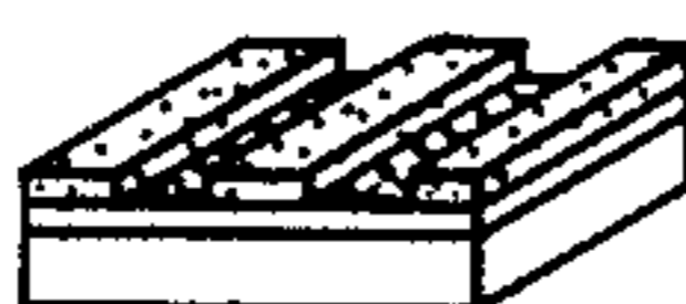
CONDUCTIVE COPPER TRACKS ETCHED
