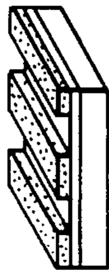
FIG. 3d RESIST DEVELOPED
