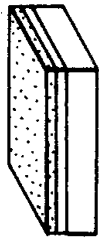
FIG. 3b COATED WITH RESIST
