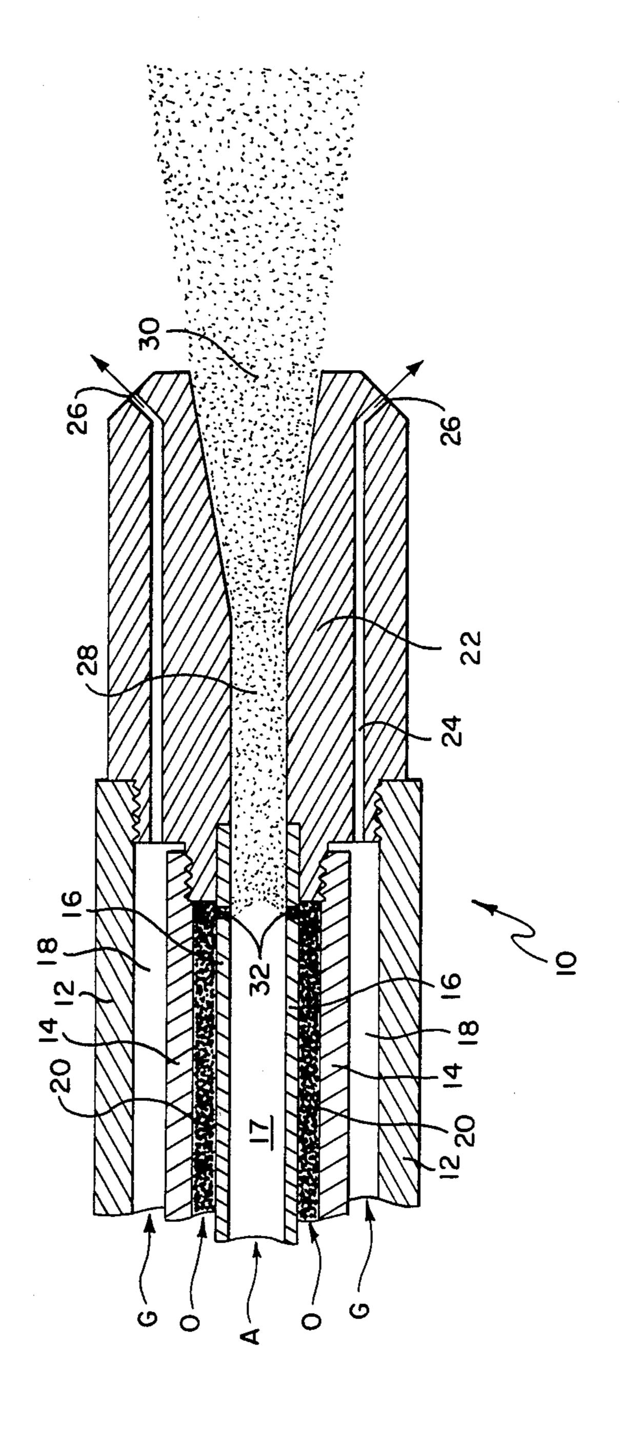
into small droplets which are discharged as a fine spray through a discharge orifice into the reactor for vaporization and carbon black formation. Preferably, a plurality of feedstock oil outlets are positioned to inject the
