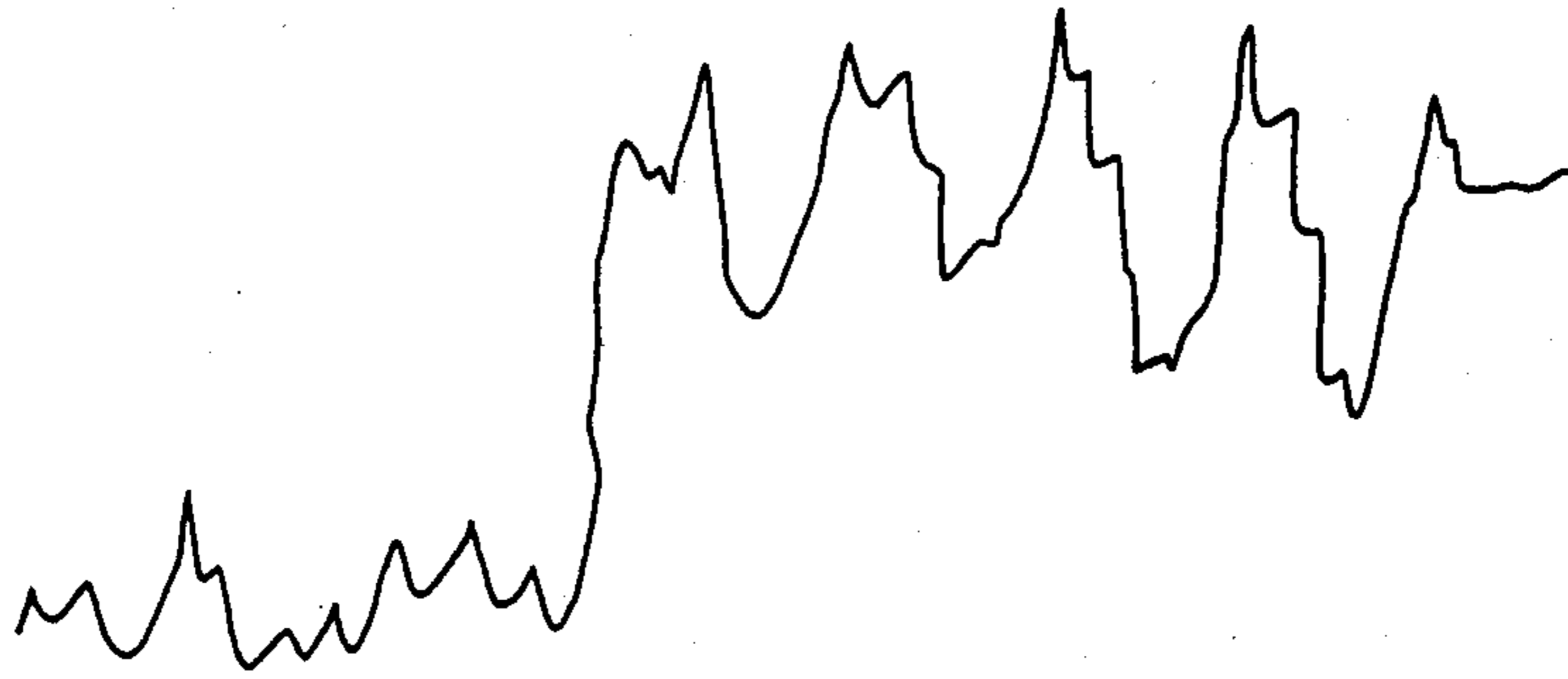
FIG. 6 TOOL BREAK ACOUSTIC SIGNATURE - TYPE 2
