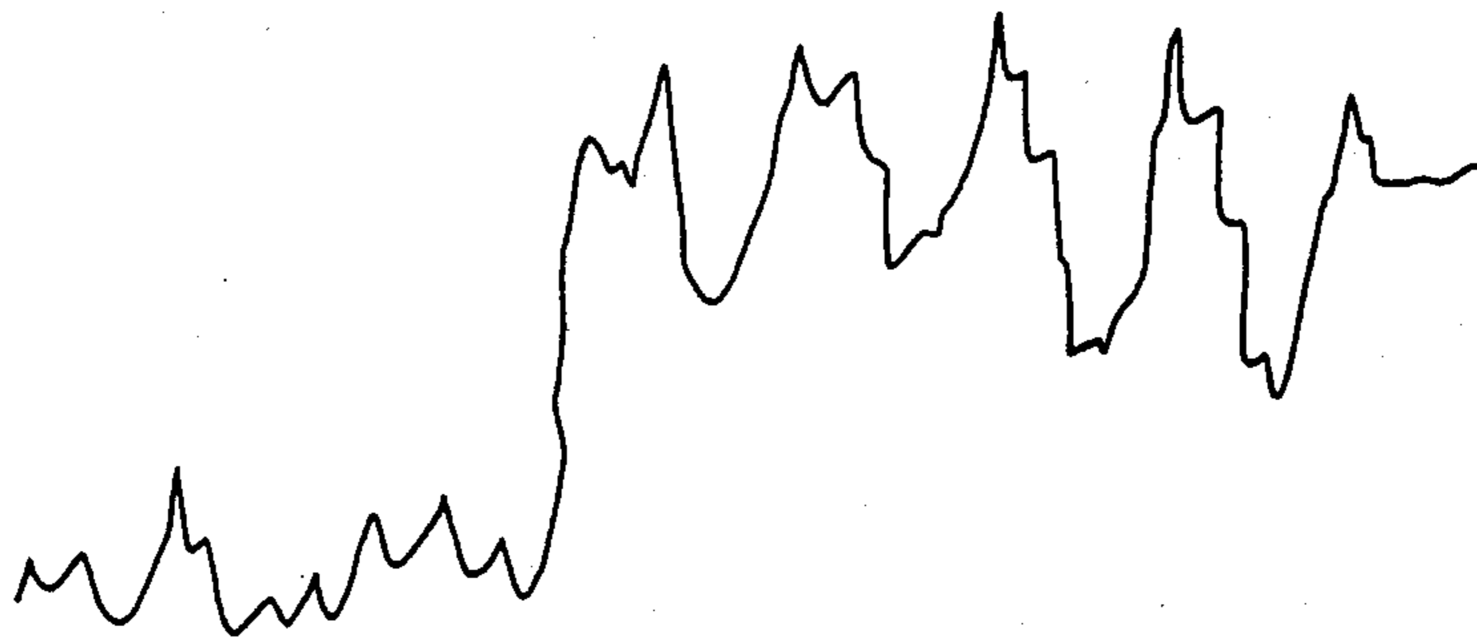
FIG. 6 TOOL BREAK ACOUSTIC SIGNATURE - TYPE 2
