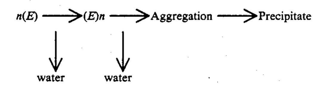
It has been found that the addition of starch (S) either to the extract of enzyme or during concentration of the enzyme circumvents the insolubilization of the enzyme at high concentrations, as represented by the following formula.
