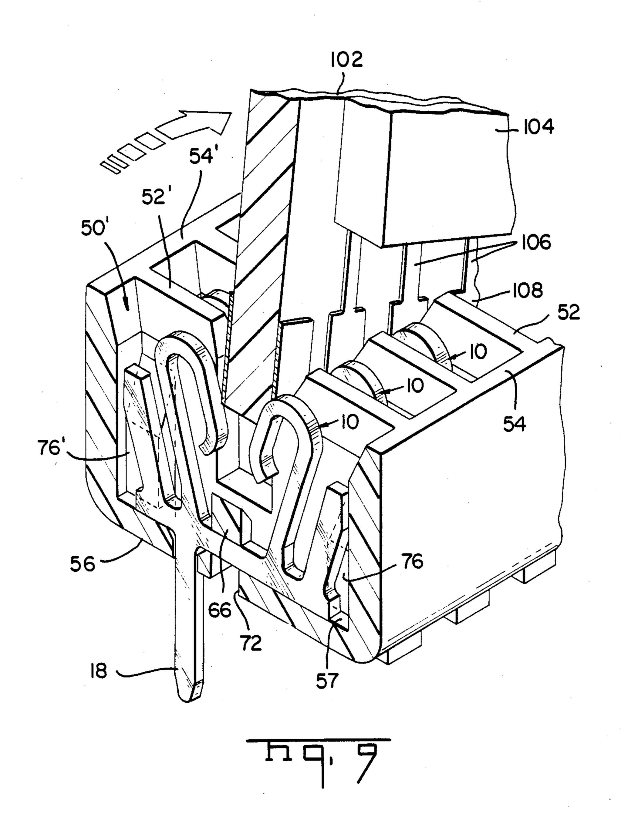
LOW INSERTION FORCE TERMINAL FOR USE WITH CIRCUIT PANEL
