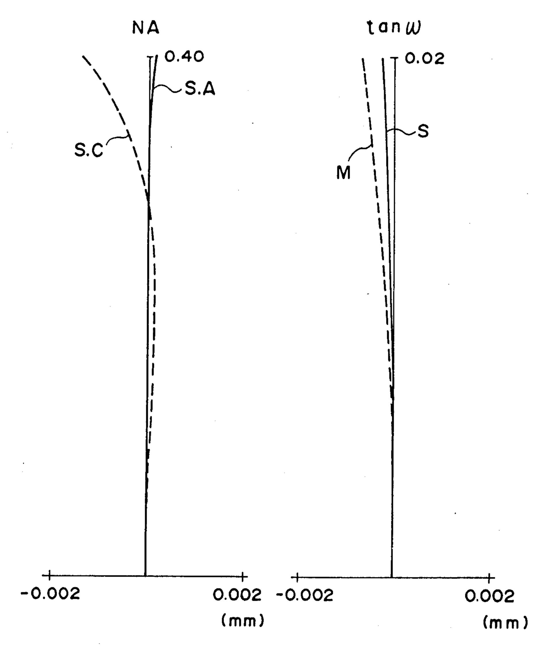
SPHERICAL ABERRATION CURVATURE OF FIELD
