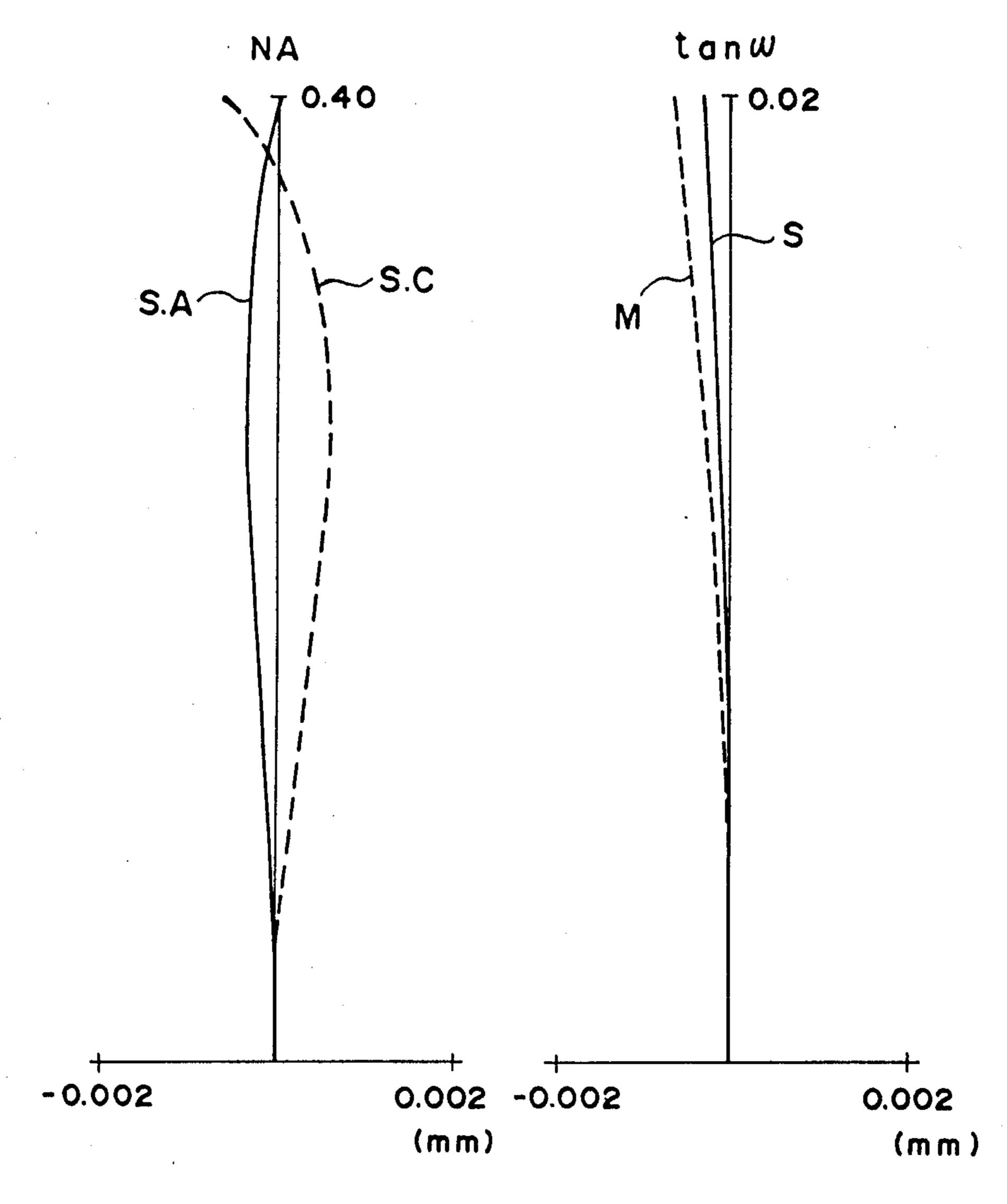
SPHERICAL ABERRATION CURVATURE OF FIELD
