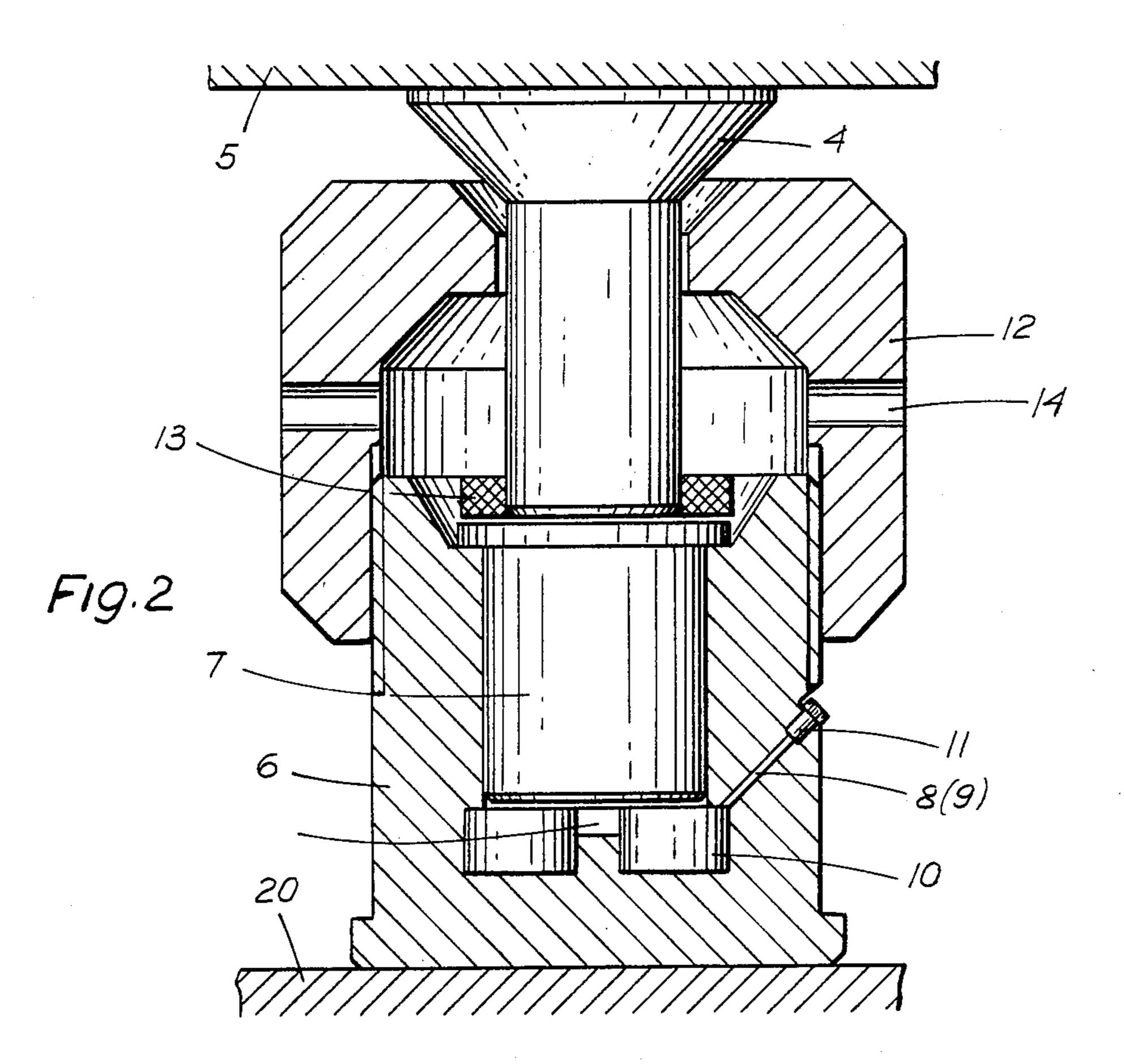
GENERATOR FOR DYNAMIC LOADING OF A MINE LINING
