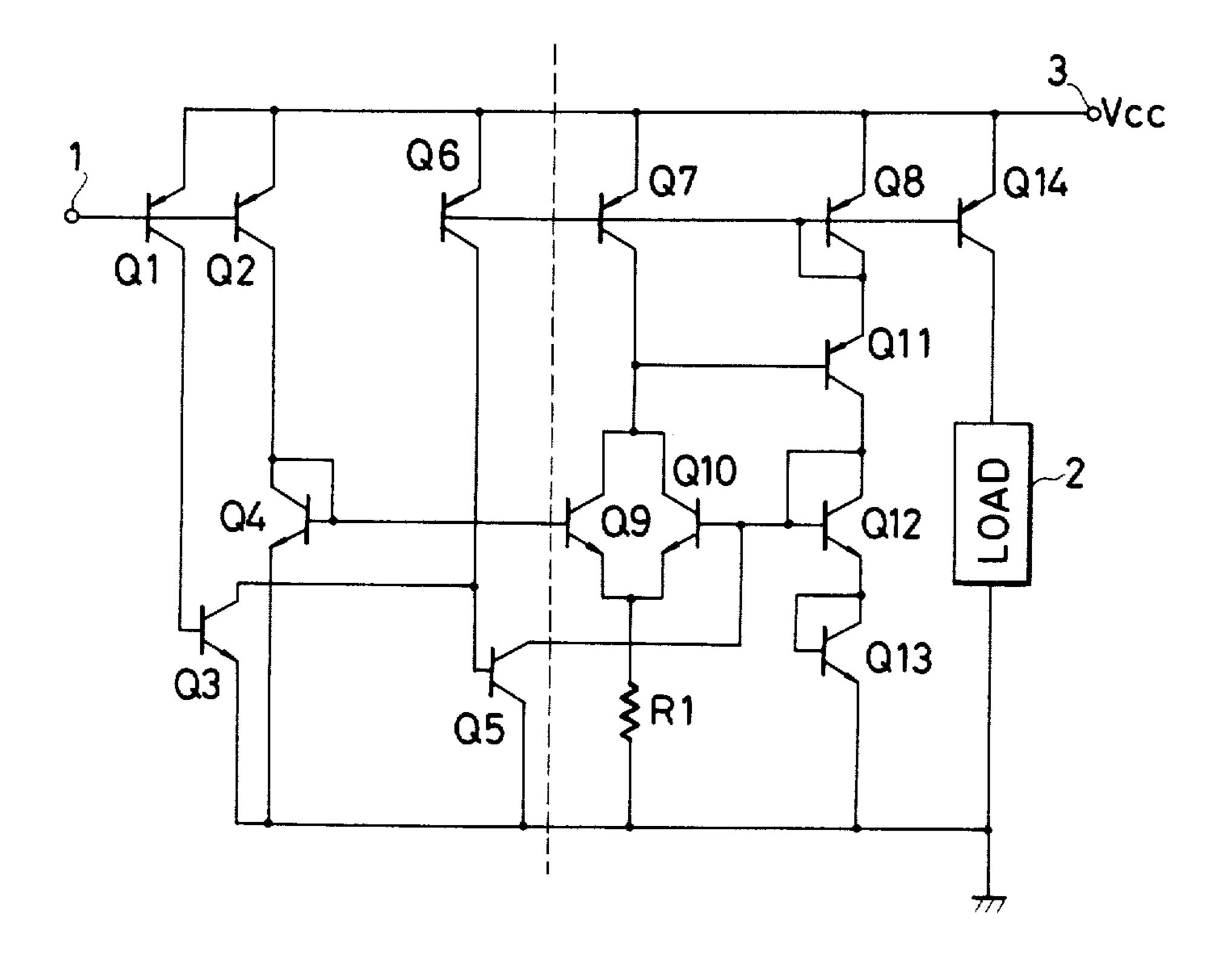
SWITCHING DEVICE HAVING A FEEDBACK MEANS FOR RENDERING A CONTROL CIRCUIT INOPERATIVE IN RESPONSE TO A CURRENT SUPPLY CIRCUIT BEING INOPERATIVE
