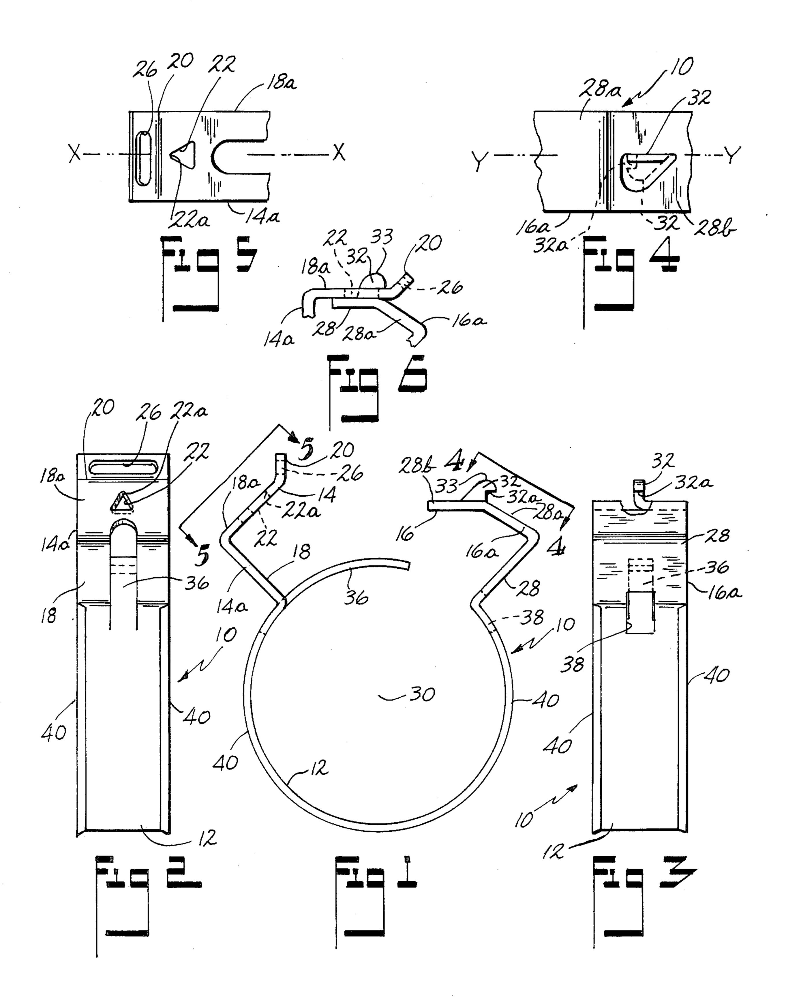
REUSEABLE CLAMP WITH AN OUTWARDLY PROJECTING EAR ON EACH OPPOSING END AND HAVING A HOOK SHAPED PROJECTION ON ONE EAR ADAPTED FOR INTERLOCKING COACTION WITH AN OPENING IN THE OTHER EAR
