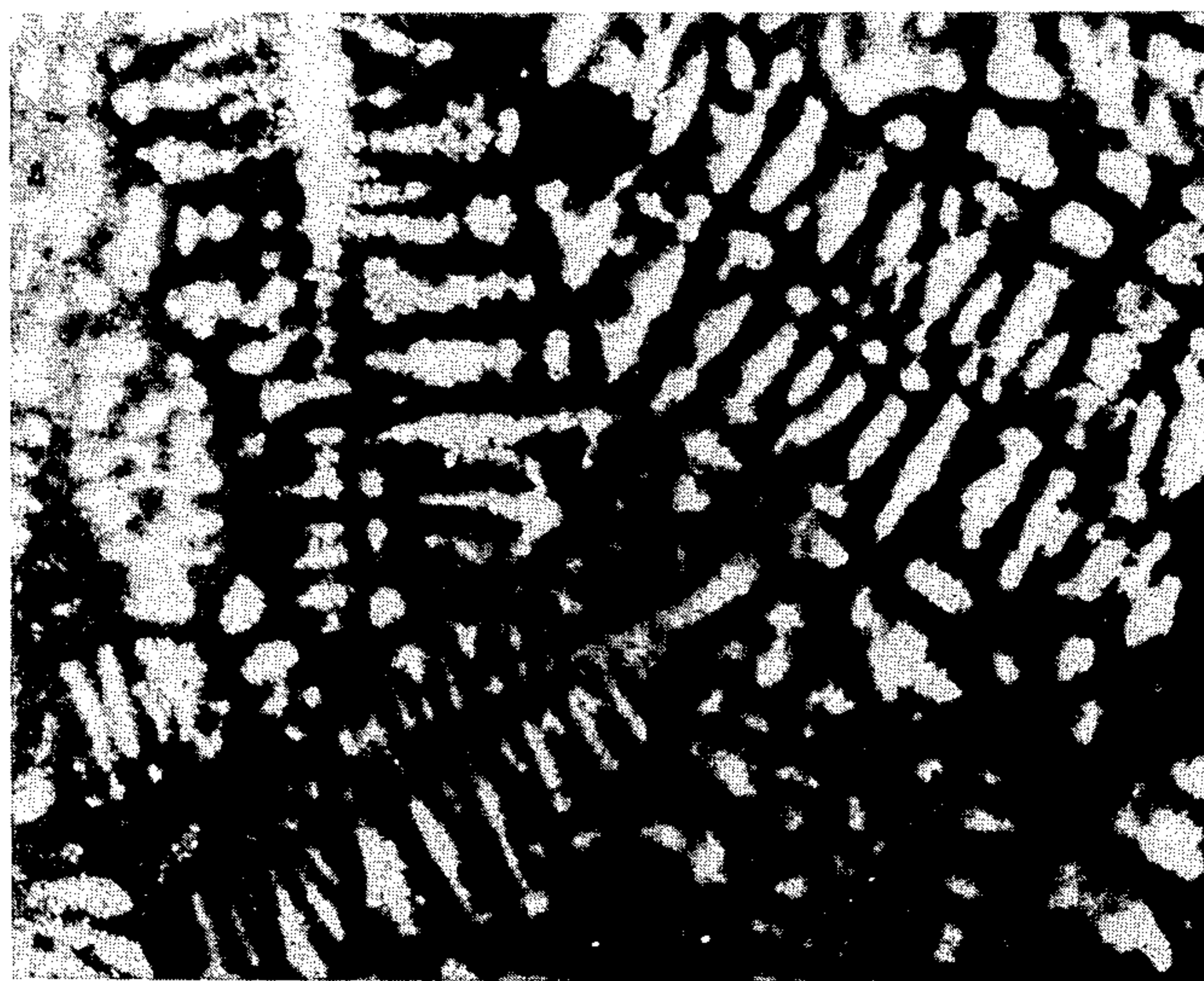
LIGHT MICROGRAPH OF SOLIDIFICATION STRUCTURE OF SPECIMEN P-2 (90.5V-9.5Ti), 256X
