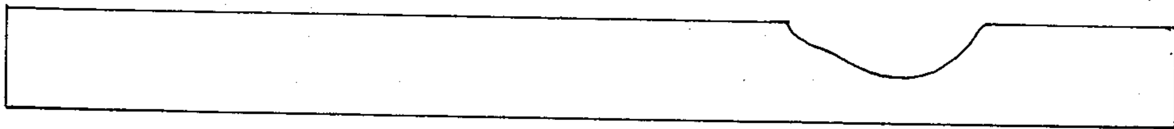
FIG. 2 BORE SURFACE WITH "BASE POROSITY" BEFORE THE BREAK-IN FINISH IS APPLIED.
