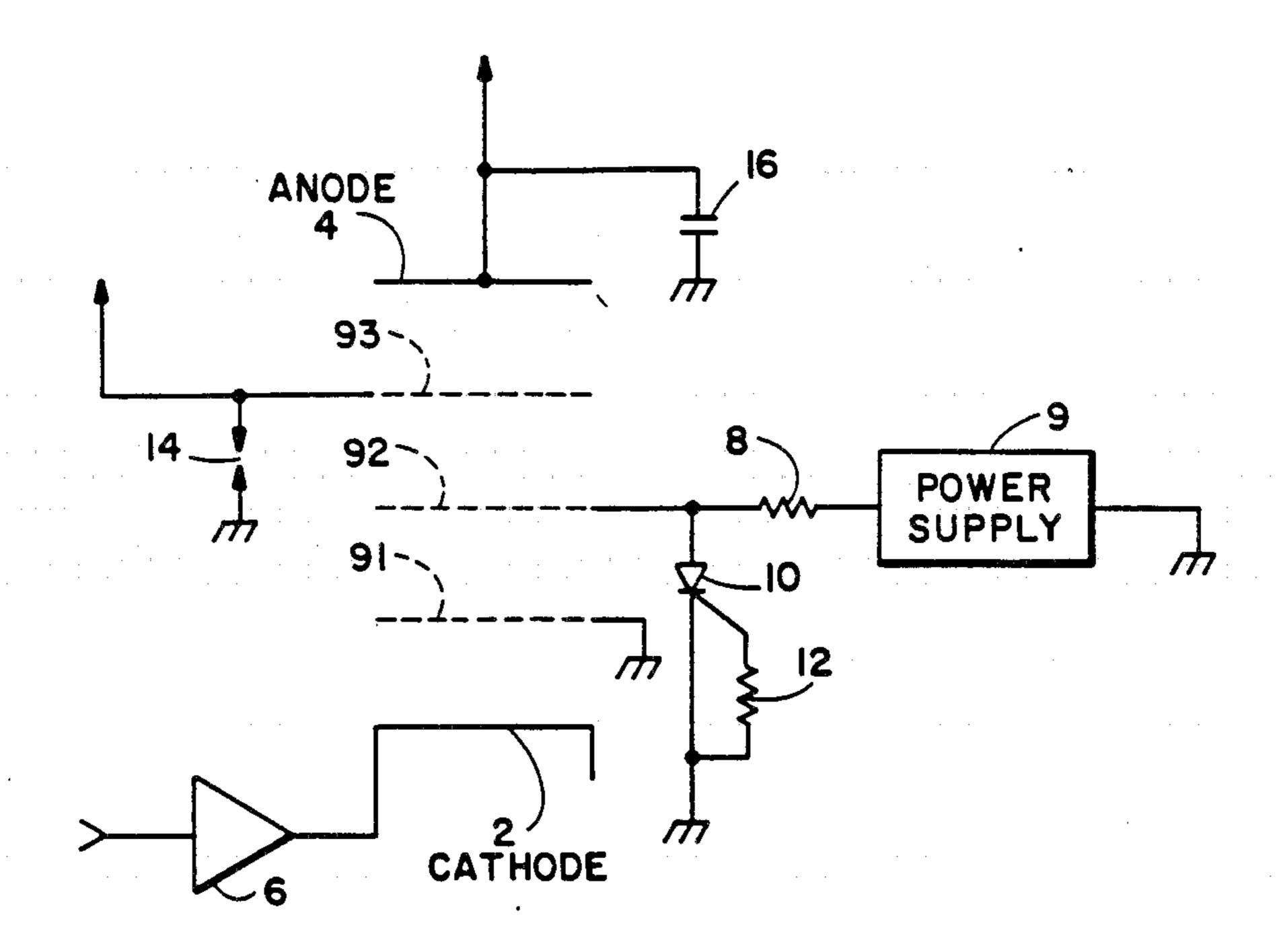
CIRCUIT ARRANGEMENT FOR PROTECTING A CRT AND ASSOCIATED CIRCUITRY FROM DAMAGE DUE TO ARCING
