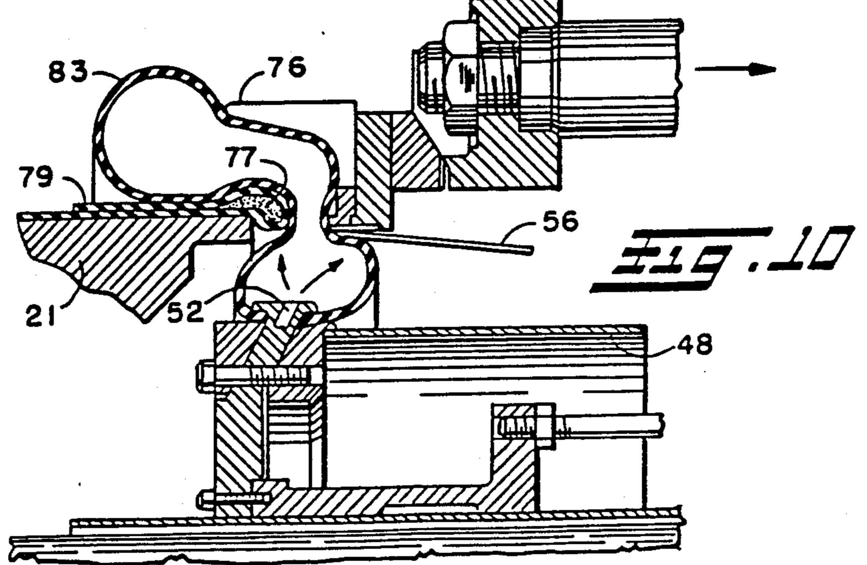
seen in applicant's U.S. Pat. No. 4,343,671 which also shows alternative usage of a dual bladder turn-up assembly.
