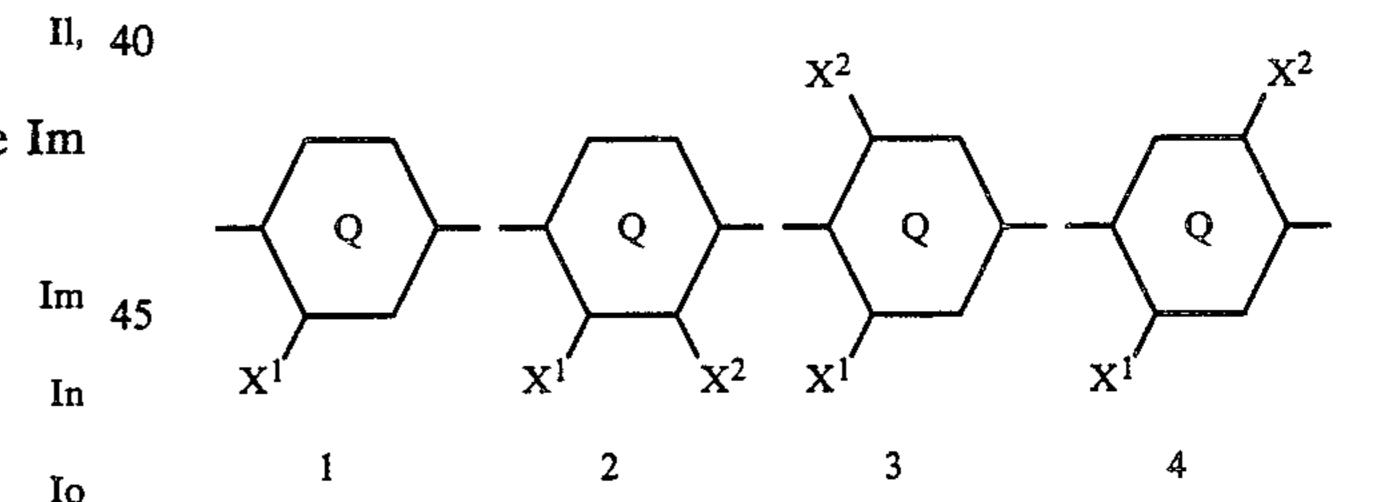
Ip 50 wherein the ring Q is a 1,4-phenylene group (structures 1 to 4), a pyrimidine-2,5-diyl group (structures 1 and 3) or a pyridazine-3,6-diyl group (structures 1 and 2), and X<sup>1</sup> and X<sup>2</sup> are each F and/or Cl and/or CH<sub>3</sub> and/or CN. In the case of the unsymmetric structures 1 to 4, formula I also includes their mirror images. The lateral substituents on the pyrimidinyl and pyridazinyl groups are in all
