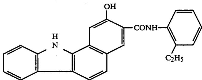
and 0.86 g of triethanolamine in 30 ml of DMF at lower than 0° C. to carry out reaction for 5 hours. Then, the reaction produced was filtered off and washed with water and then with acetone and DMF to yield 0.83 g of the objective pigment. m.p. 337° C. (decomp.)
