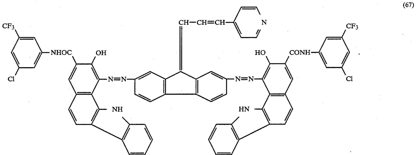
The electrophotographic photoreceptor of this invention has a light-sensitive layer containing the bis-azo pigment represented by the general formula [I] or [II] and the bis-azo pigment may be used in various man-
