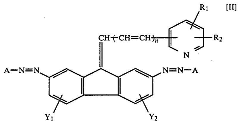
wherein Y<sub>1</sub> and Y<sub>2</sub> each represent a hydrogen atom, a halogen atom, an alkyl group or an alkoxy group, R<sub>1</sub> and R<sub>2</sub> each represent a hydrogen atom, an alkyl group, an alkoxy group or a group of atoms necessary to form a condensed ring by combination of them, A represents a coupler residue necessary to produce an azo pigment and n is 0 or 1.
