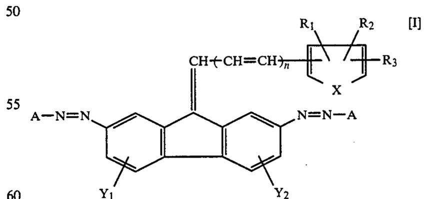
wherein X represents -O-, -S- or >N-R<sub>4</sub> where R<sub>4</sub> represents a hydrogen atom, an alkyl group or an aralkyl group, R<sub>1</sub>, R<sub>2</sub> and R<sub>3</sub> each represent a hydrogen atom, an alkyl group, an alkoxy group, an aryl group or two of R<sub>1</sub>, R<sub>2</sub> and R<sub>3</sub> being a group of atoms necessary to form a condensed ring by combination of them, Y<sub>1</sub> and Y<sub>2</sub> each represent a hydrogen atom, a halogen
