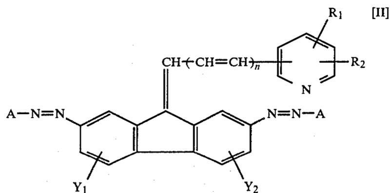
wherein  $Y_1$  and  $Y_2$  each represent a hydrogen atom, a halogen atom, an alkyl group or an alkoxy group,  $R_1$  and  $R_2$  each represent a hydrogen atom, an alkyl group, an alkoxy group or a group of atoms necessary to form a condensed ring by combination of  $R_1$  and  $R_2$ ,  $A$  represents a coupler residue necessary to produce an azo pigment and  $n$  is 0 or 1.
