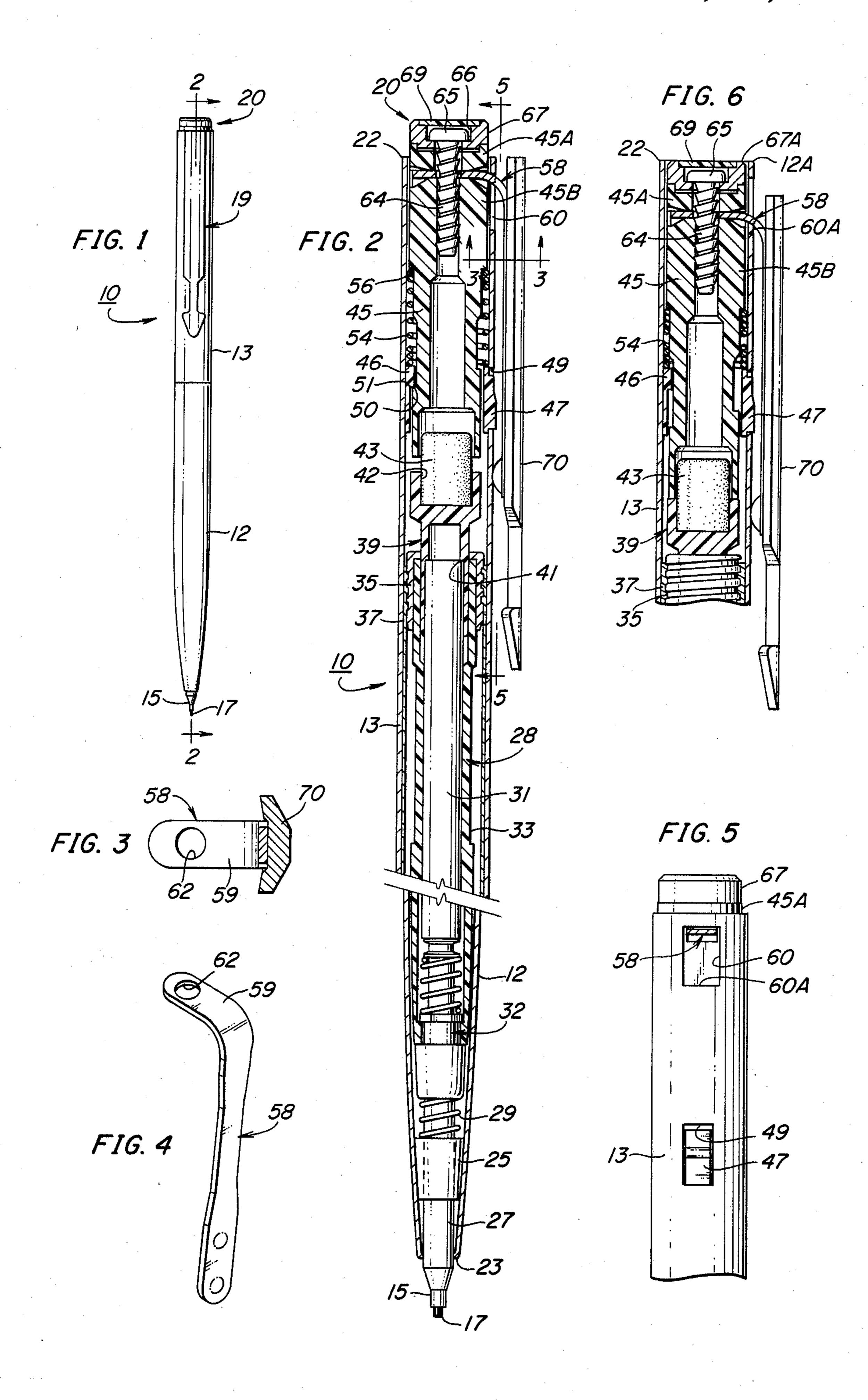
CONTINUOUS FEED MECHANICAL PENCIL WITH PUSH BUTTON LEAD FEED ACTUATOR
