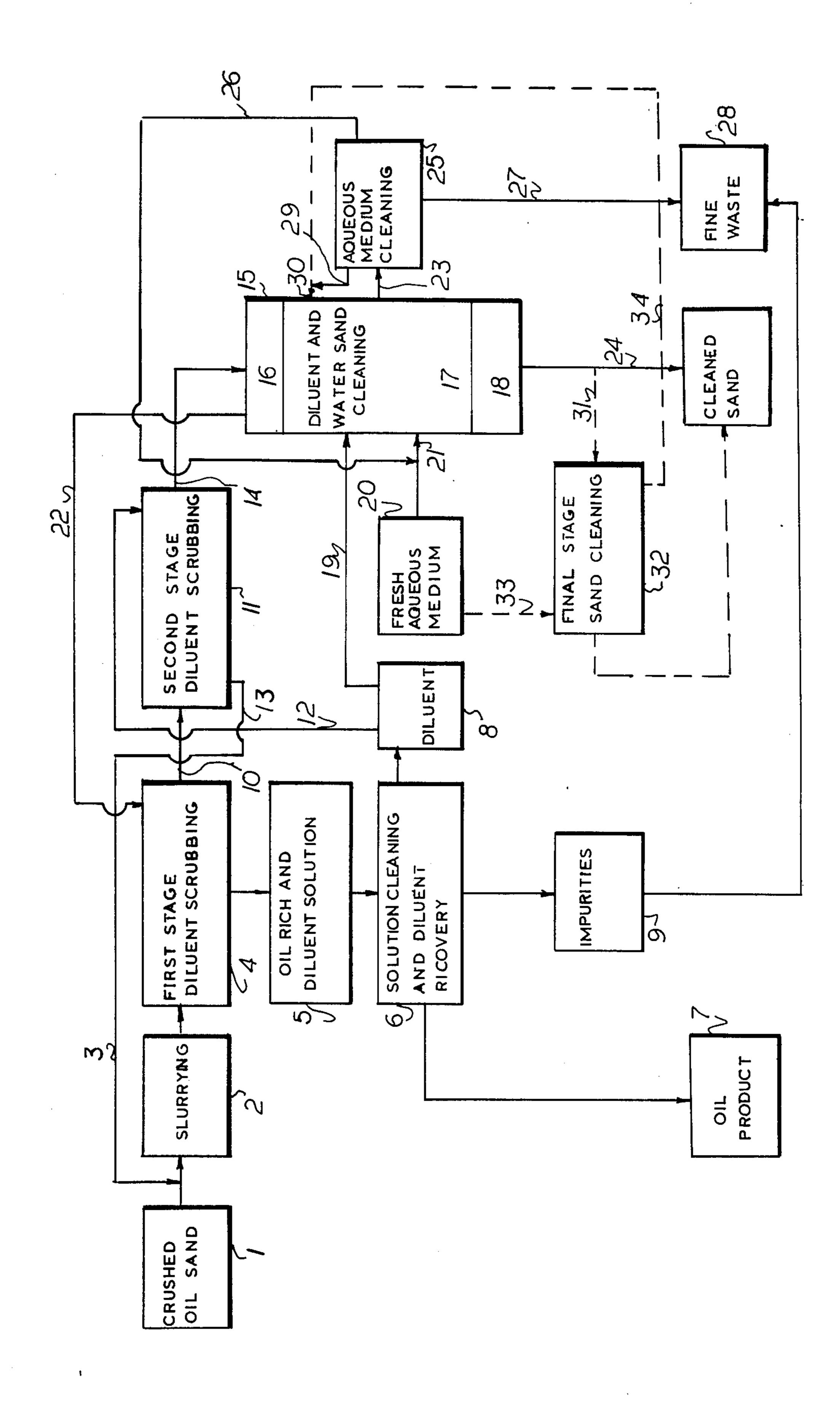
PROCESS OF ORGANIC MATERIAL EXTRACTION FROM BITUMINOUS SANDS OR OIL BEARING SANDS
