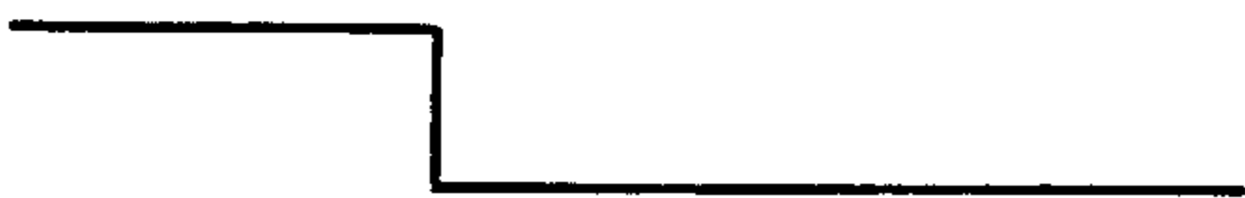
FIG. 4E 306Z OUTPUT IN THE CASE OF HIGH PASS FILTER CHARACTERISTIC
