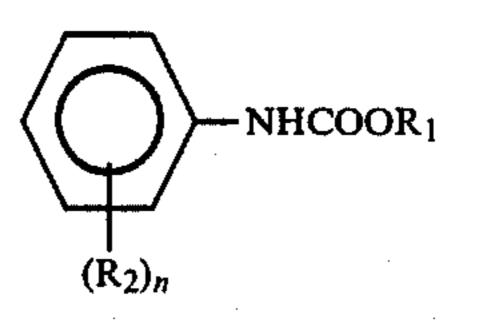
wherein  $R_1$  is an alkyl, an alicylic or an aromatic group; each  $R_2$  is individually selected from hydrogen, alkyl, halogen, nitro or alkoxyl and n is 0 to 4.
