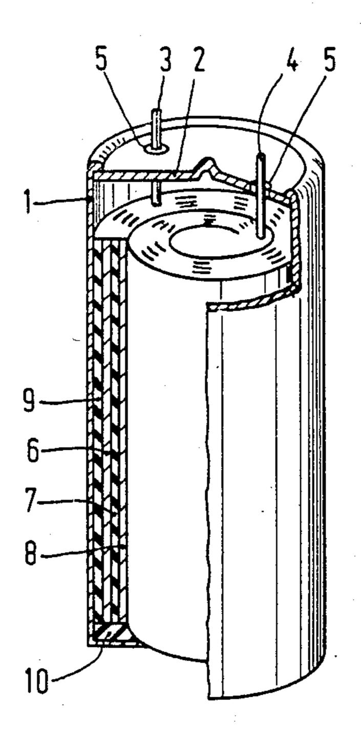
A further object of the invention is to provide an electrochemical cell having a high power density at low operational temperatures.
