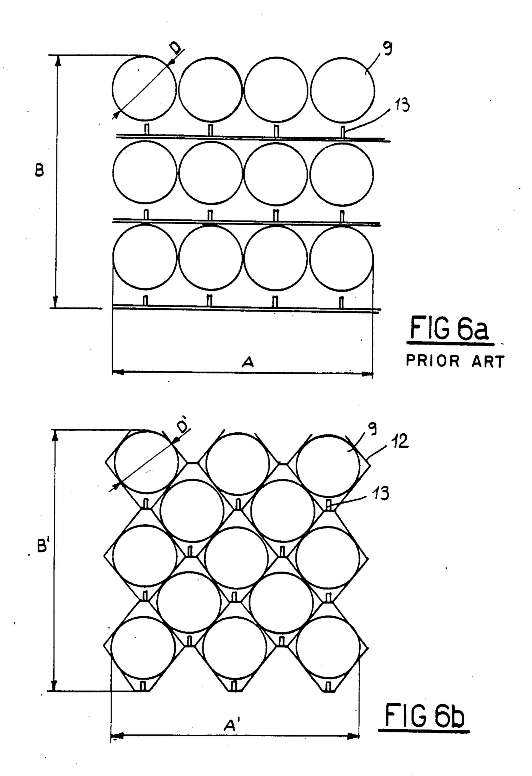
CREEL STRUCTURE TO SUPPORT WARP AND WEFT YARN DELIVERY BOBBINS IN LOOMS
