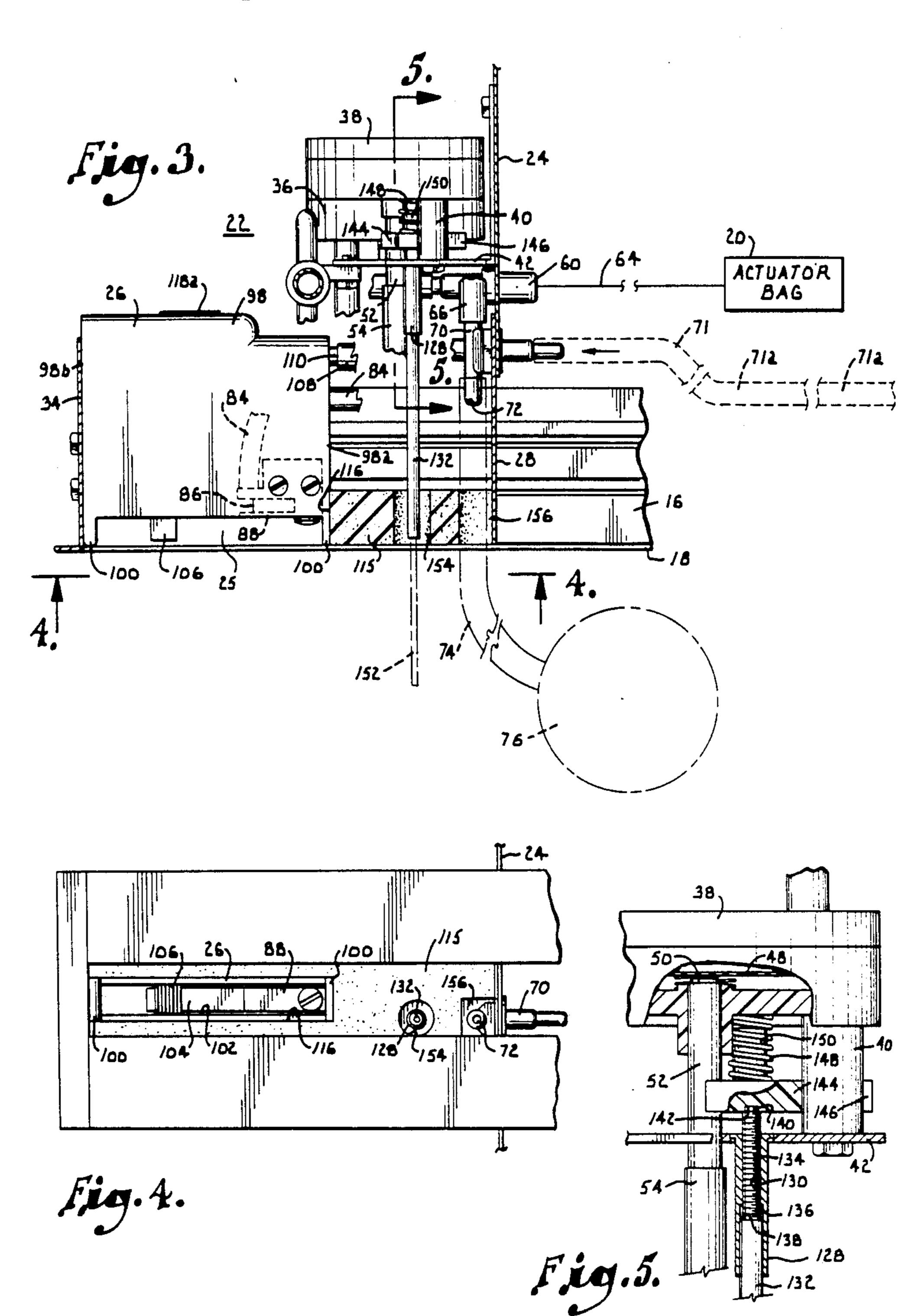
CONTROL INSTALLATION FOR VARIABLE **VOLUME AIR DIFFUSERS**
