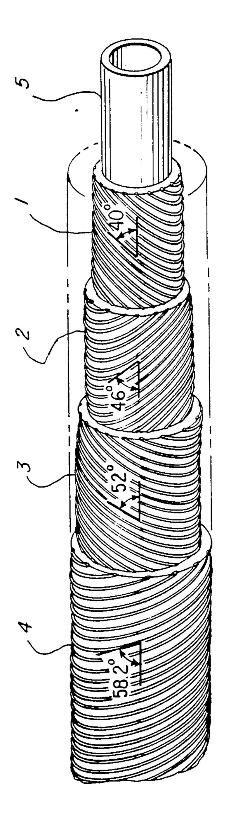
VARIABLE MODULUS FILAMENT WOUND PRESSURE TUBE
