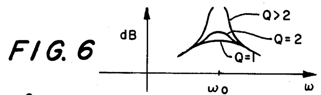
Since  $\frac{s^2}{\omega_0} = -1$  when  $s = j\omega_0$ , the sinusoidal gain at the center frequency is
