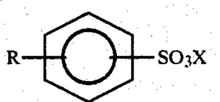
where R is a linear alkyl radical having from about 10 to 18 carbon atoms and X is a cation as previously defined in this specification, can also be substituted in part, for the alcohol sulfate or ethoxylated alcohol sulfate of the invention composition. A typical formula is:
