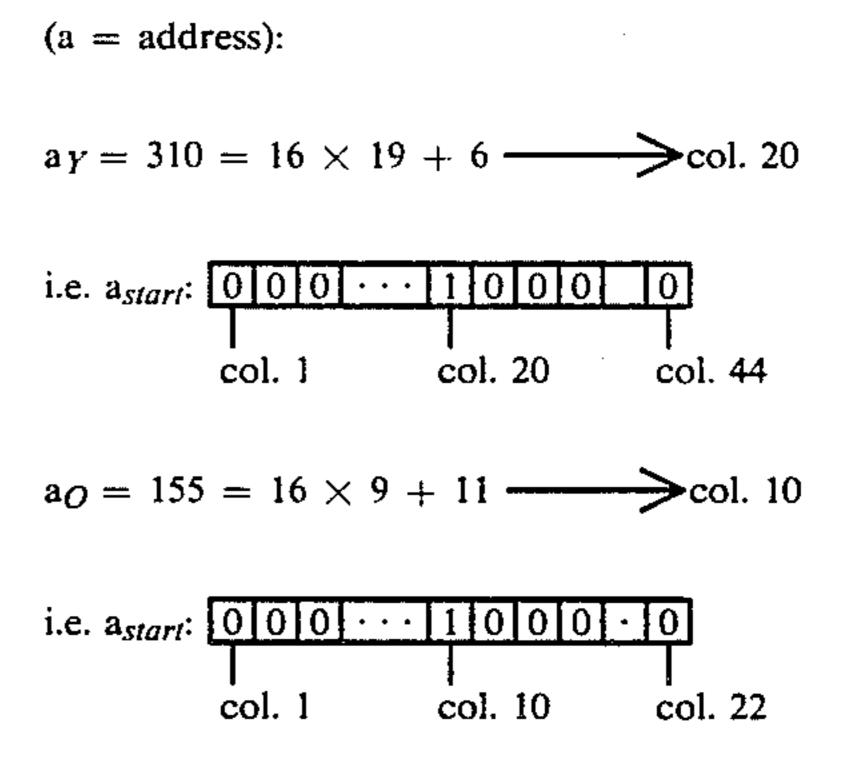
In the luminance mode, the 44 outputs of the register 141 are used to address the memory Y. Because of the fact that there are two memories Y operating in the write or read mode, each formed by two memory portions, two addressing circuits are required for each memory Y, one for the high portion the other for the low portion.
