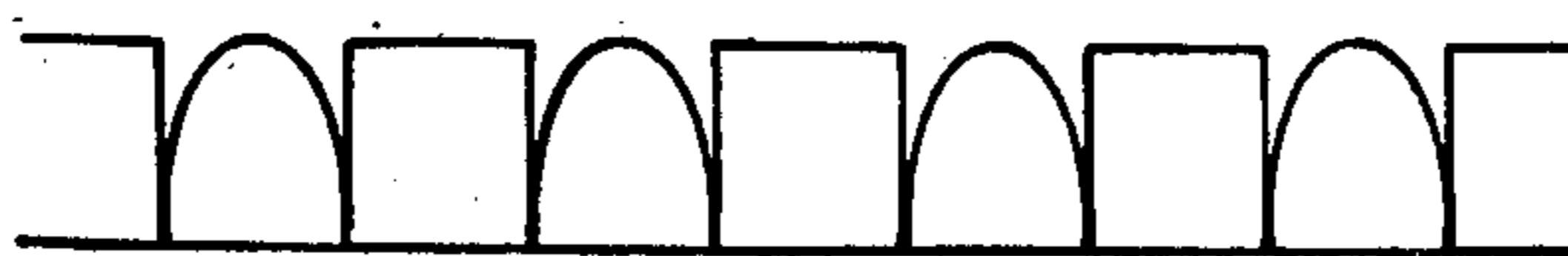
FIG-4 MODIFIED AC REFERENCE SIGNAL
